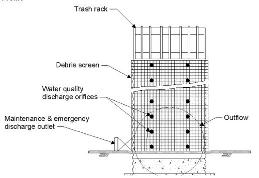
FIGURE 3: MULTIPLE ORIFICE OUTLET RISER
