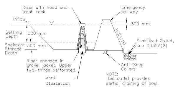
FIGURE 2: MULTIPLE ORIFICE DESIGN NOT TO SCALE
