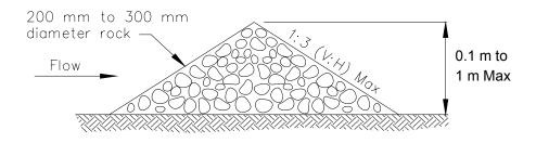
TYPICAL ROCK CHECK DAM SECTION
