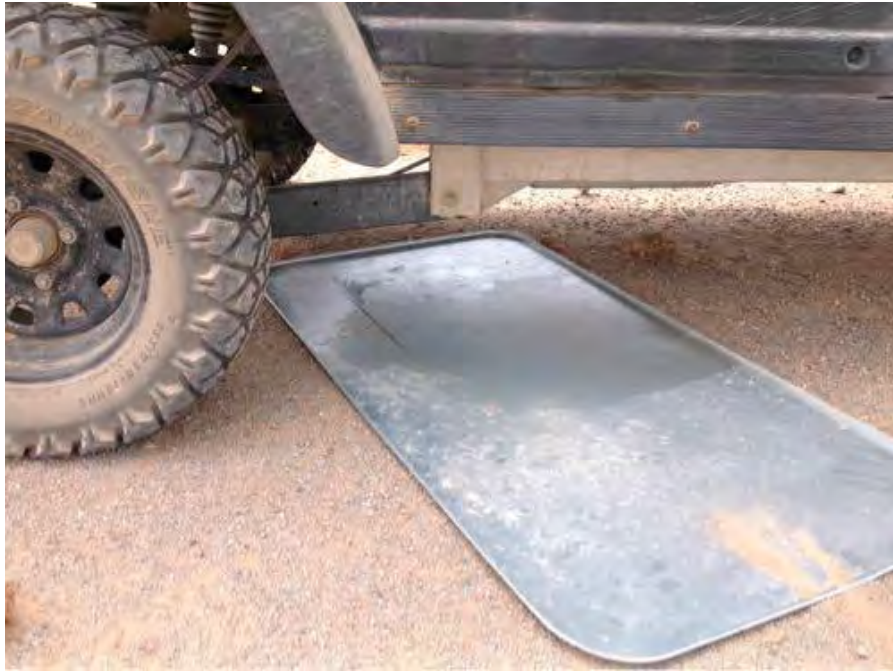
Photo 3: DF Bio-8: Minimize Spills of Hazardous Materials Drip pan placed beneath equipment in Unit 2; August 6, 2015
