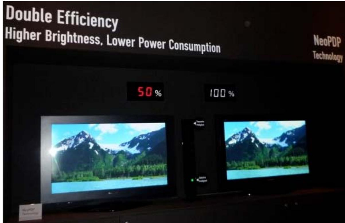
The TV left is the plasma display developed with the "high luminance efficiency technology" and the TV on the right is the 2007 model. Same brightness using half the power.
