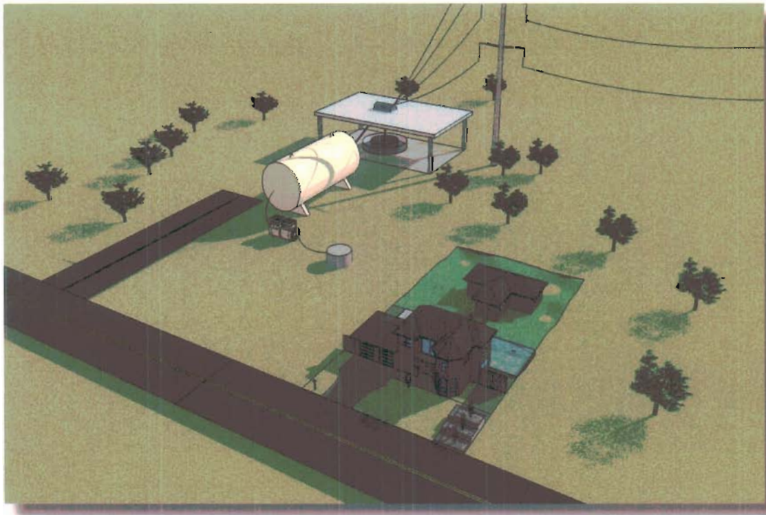
(fig. 2a - A CAD drawing showing a Nereus Compressed Air System storing and releasing energy for a residential area.)
