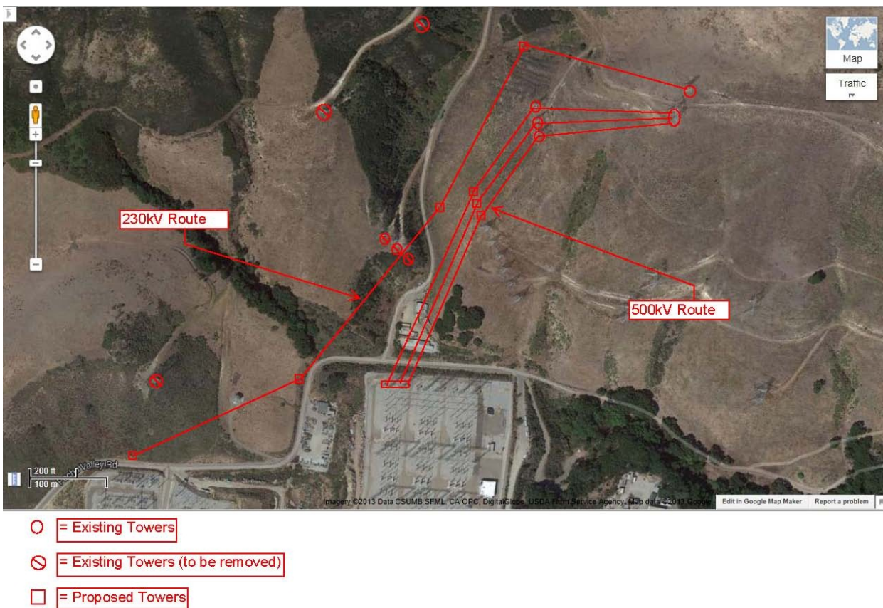
Figure 4.3-7. Existing 230 kV and 500 kV Power Line Rerouting
