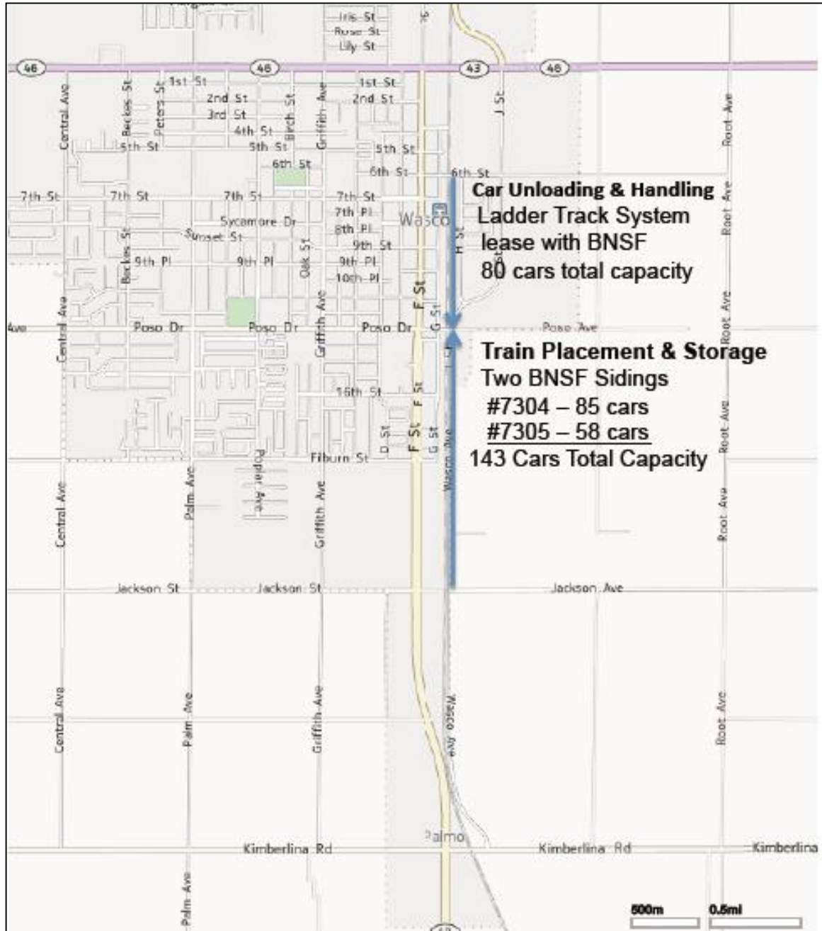
WASCO COAL TERMINAL - A 240 BNSF Train Handling / Storage Sidings
