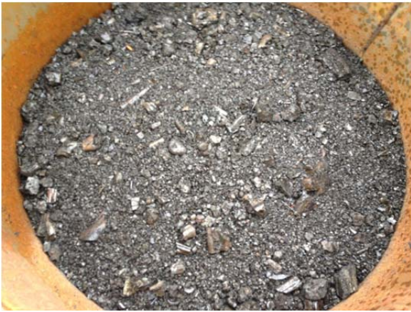
Figure 2A. Raw slag in shipment container.
