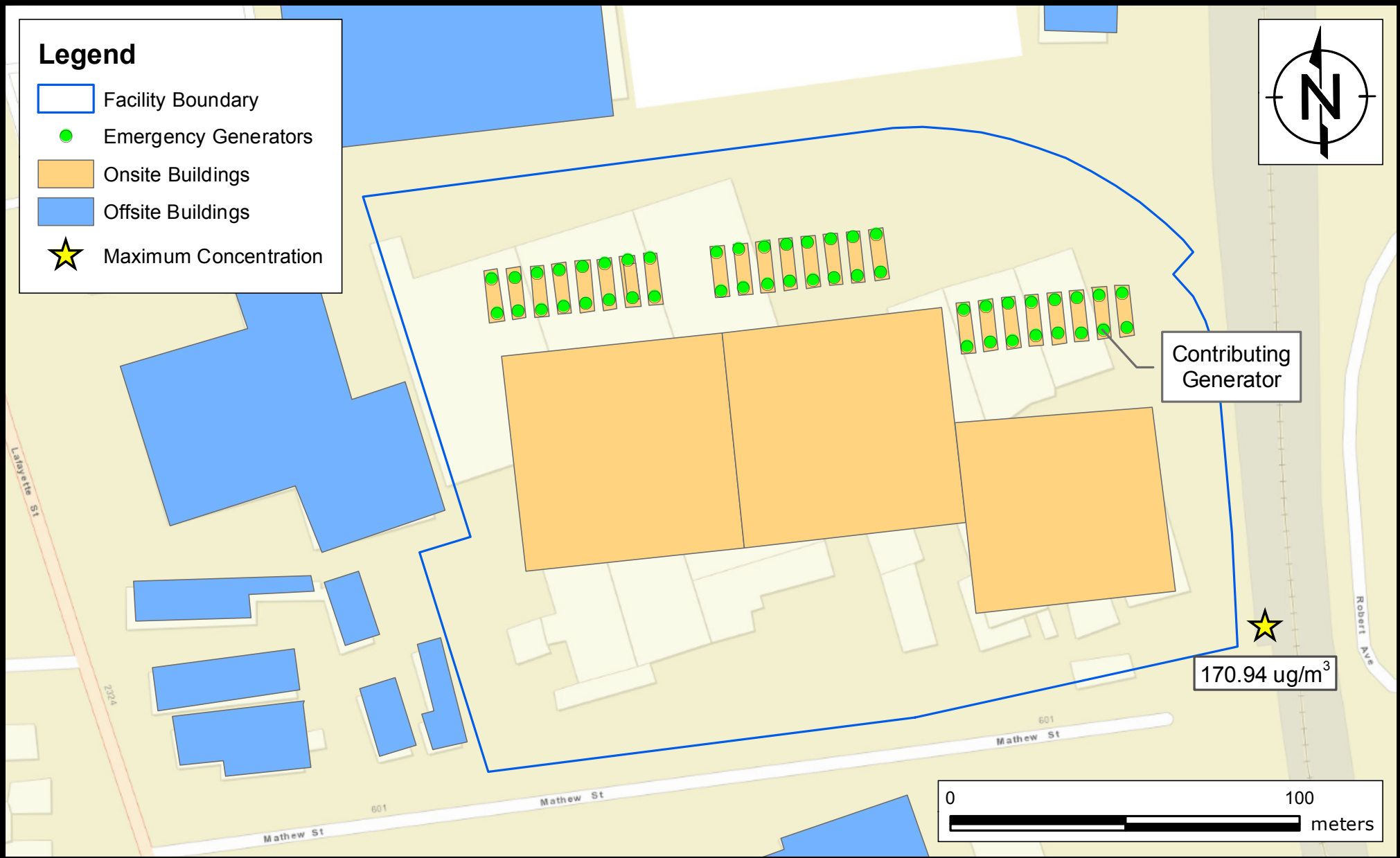
Maximum 1-Hour NO2 Concentration (NAAQS) and Contributing Generator Vantage McLaren Campus Sanat Clara, California
