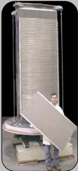
Individual fuel cell & 350 kW fuel cell stack
