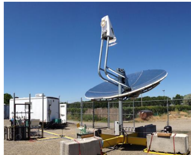
Solar Concentrator Test Stand
