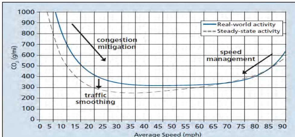
Figure 4-2: Possible Effect of Traffic Operation Strategies in Reducing On-Road CO<sub>2</sub> Emission<sup>8</sup>
