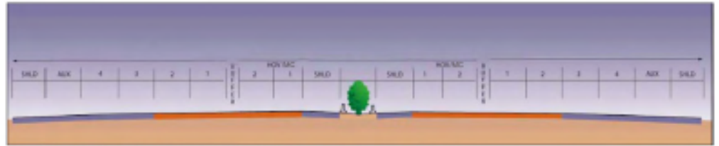
Proposed Project: 8+4 with Buffer - Eight general purpose lanes and four HOV/Managed lanes separated by 1.2m (4 ft) wide striped buffer zones
