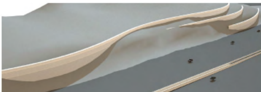
An example of terrain contoured retaining wall
