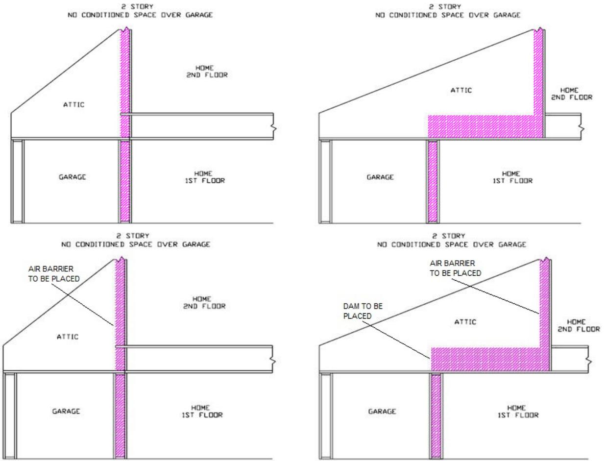
Figure RA3.5-2 Homes with No Conditioned Space Over Garage – Batt and Blanket Insulation
