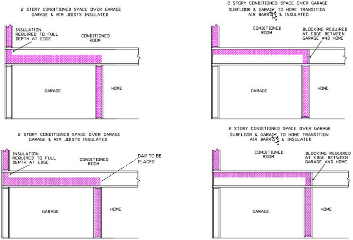
Figure RA3.5-1 Homes with Conditioned Space Over Garage – Batt and Blanket Insulation
