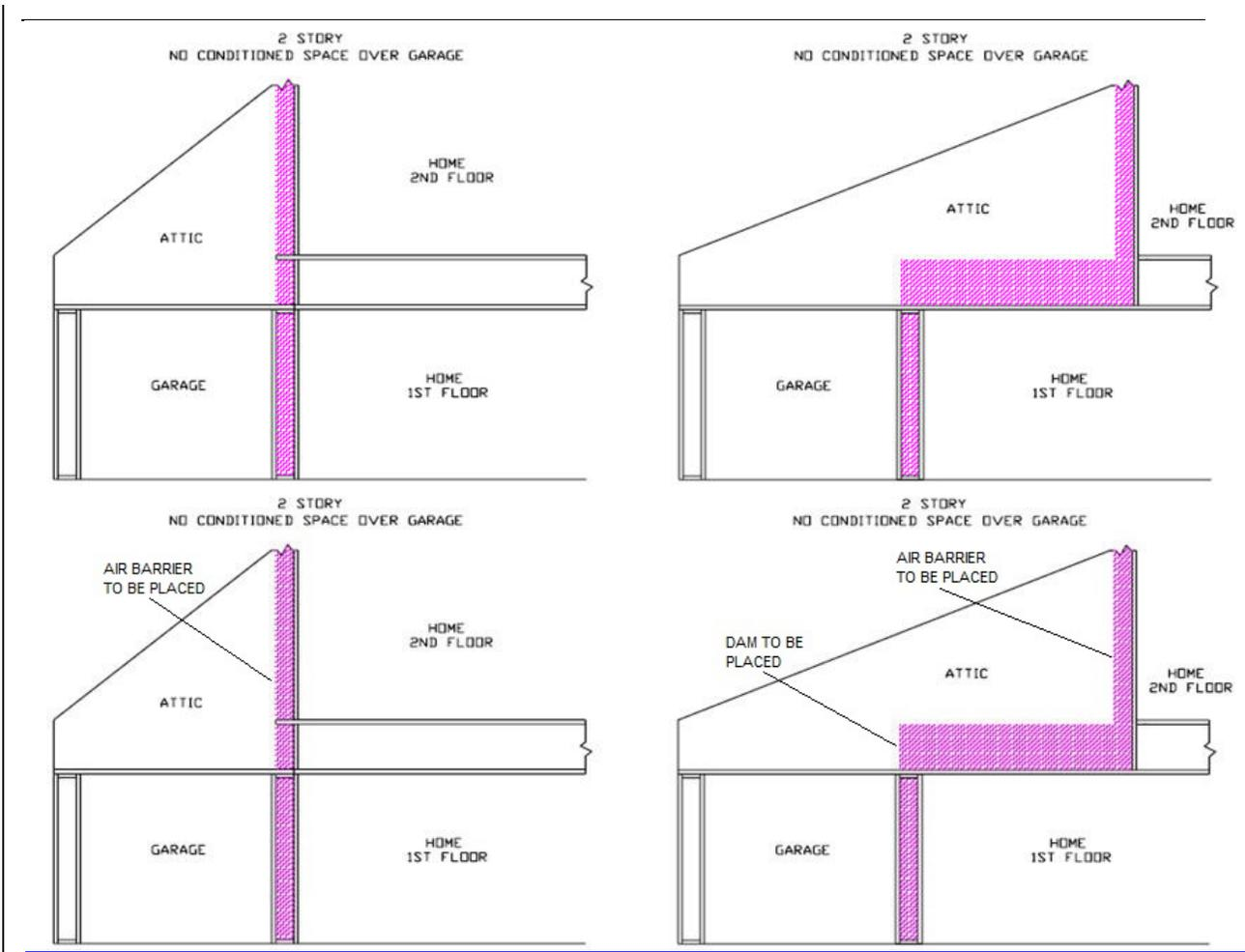
Figure RA3.5-4 Homes with No Conditioned Space over Garage – Loose Fill Insulation
