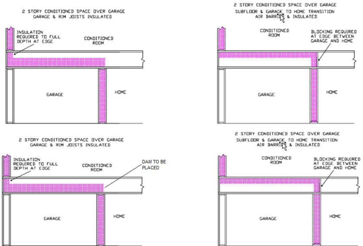
Figure RA3.5-3 Homes with Conditioned Space Over Garage – Loose Fill Insulation
