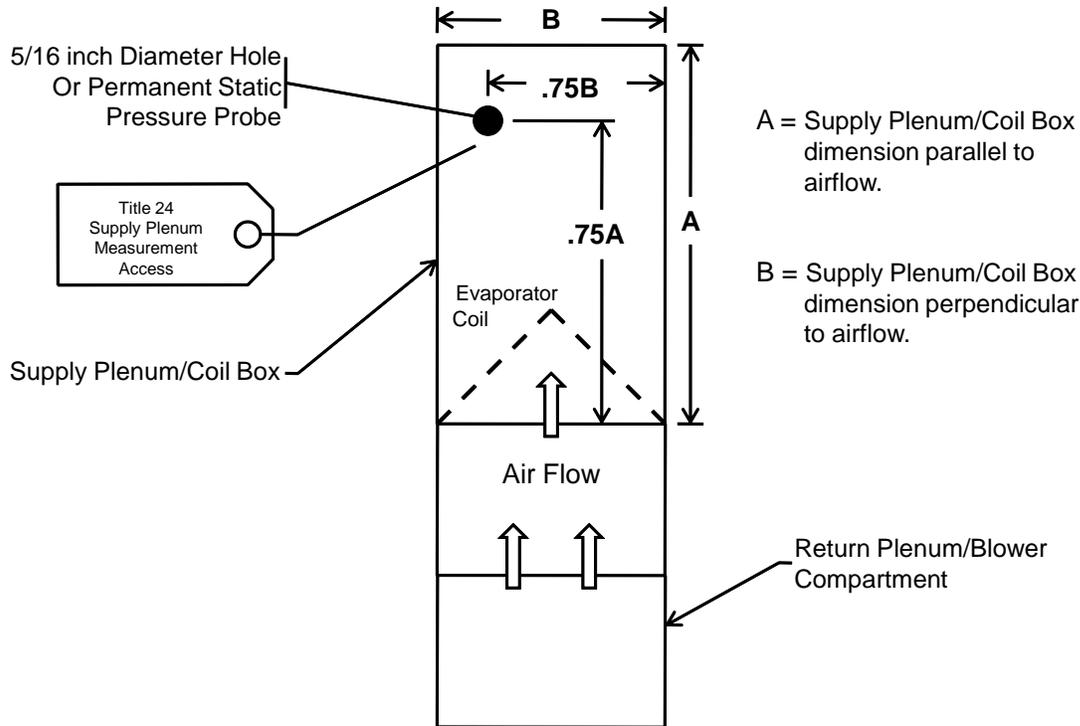
Figure RA3.3-1 Hole for the Placement of a Static Pressure Probe (HSPP)
