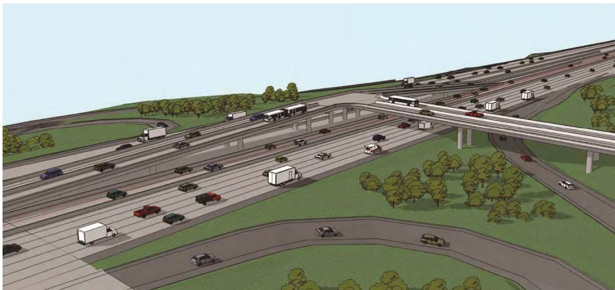
Figure 2-2.5a: Typical Overhead DAR
