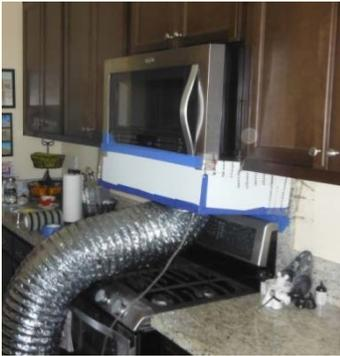
Range hood airflow measured using a capture hood and calibrated fan
