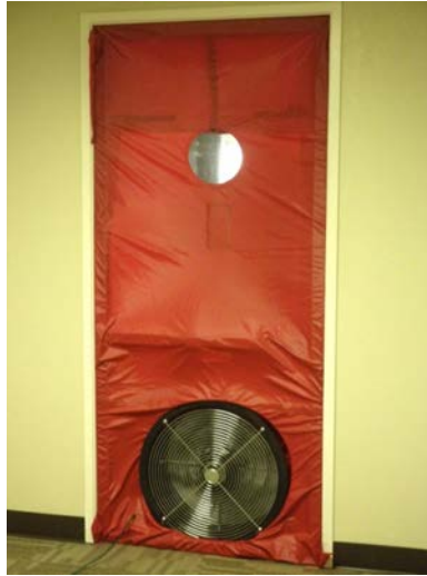
Figure 9: Blower Door Testing of a Multifamily Apartment
