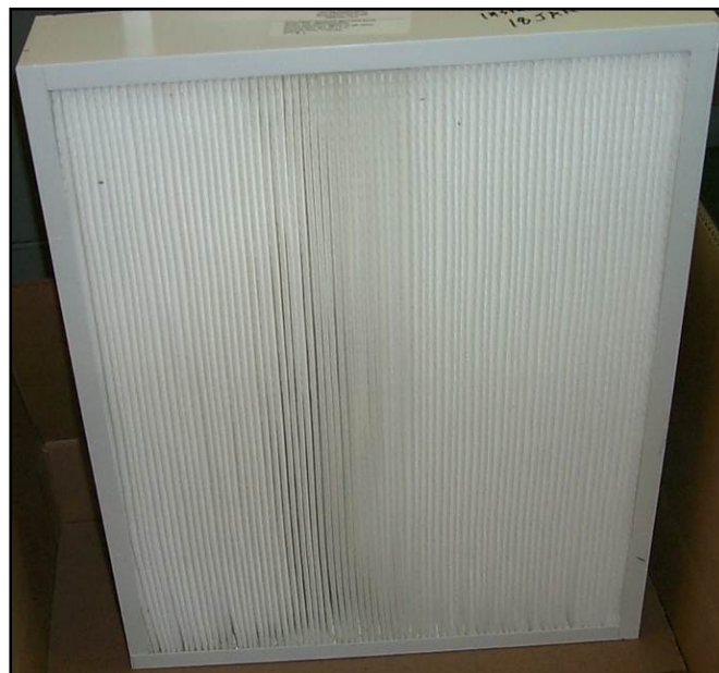
Figure 4: House 1 MERV 16 Filter
