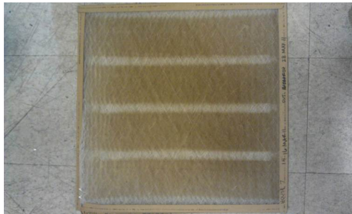
Figure 59: Ceiling Return Filter Used in House 7
