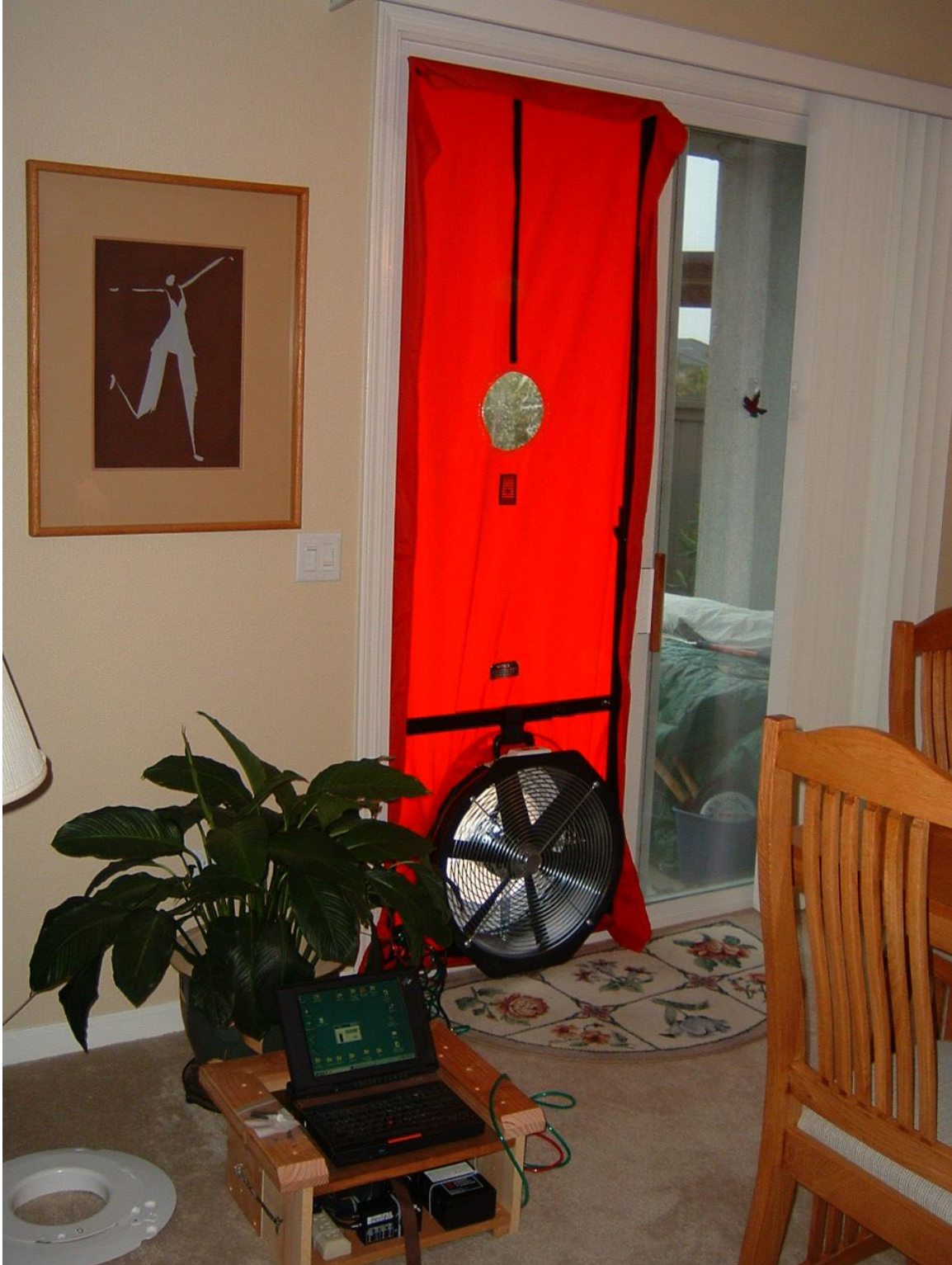
Figure 5. Pilot Home P2, Blower Door and APT installed.
