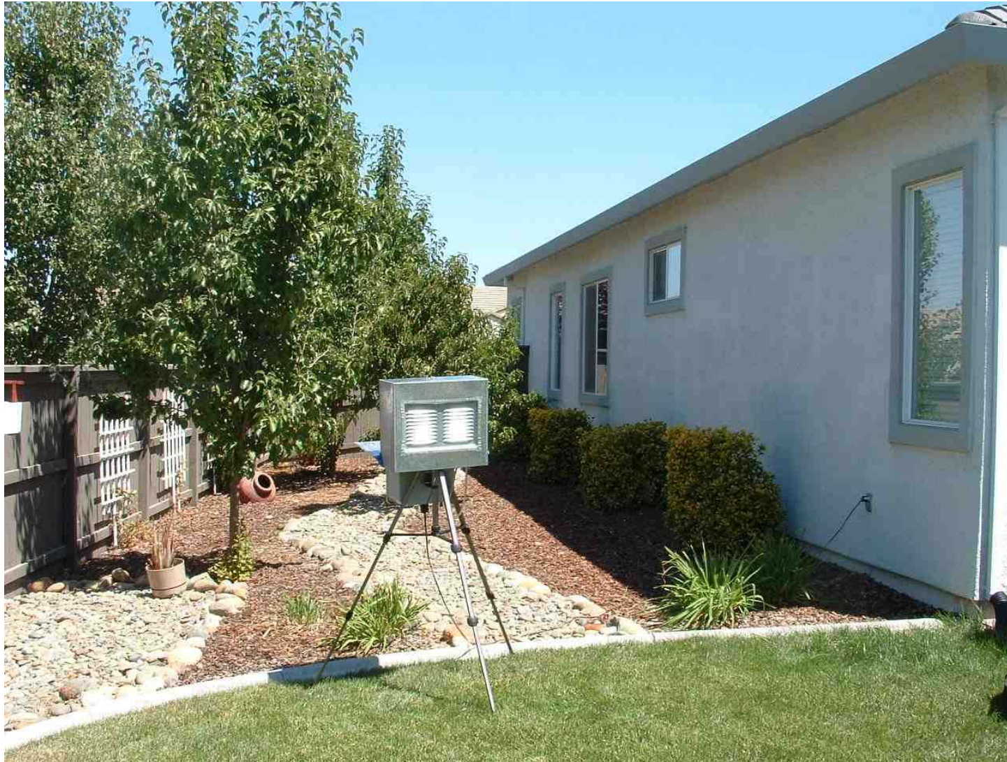
Figure 2. Outdoor air sampler for formaldehyde, VOCs, PM 2.5 , NO 2 , CO, CO 2 , temperature, and relative humidity, with outdoor radiation/rain shield.
