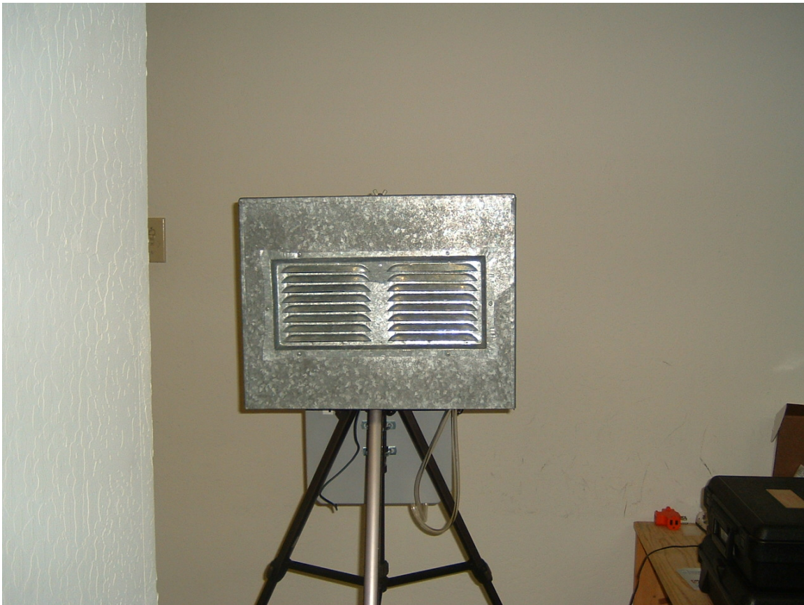
Figure 3. Close-up of air sampling rig with outdoor radiation/rain shield.
