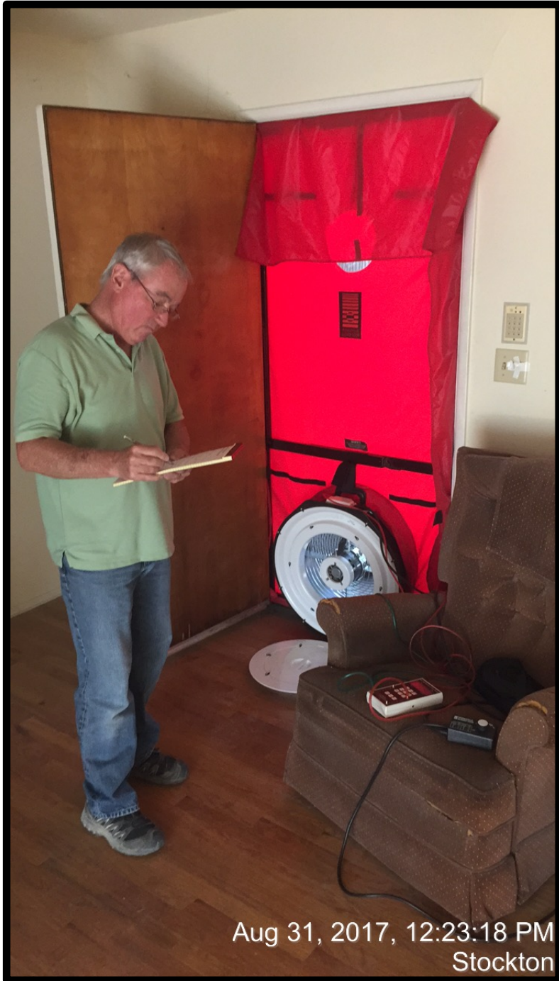
Blower Door Pressure Matching Method
