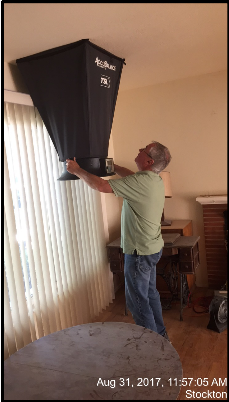
Capture Hood: Rated for use up to about 2,000 CFM
