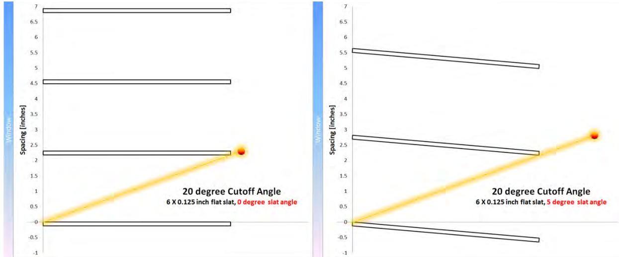
**Figure 7: Slat angles and spacing for a given cutoff**
