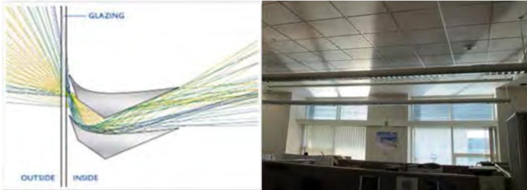
**Figure 9: LightLouver profile and field installation**
