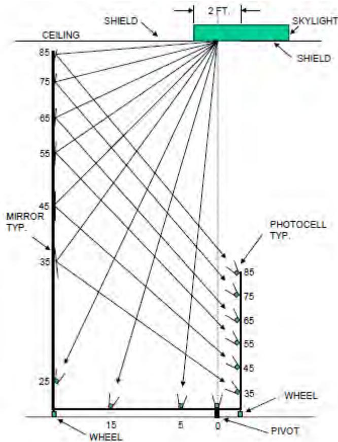
**Figure 14: PIER skylight photometric testing using a goniophotometer**
