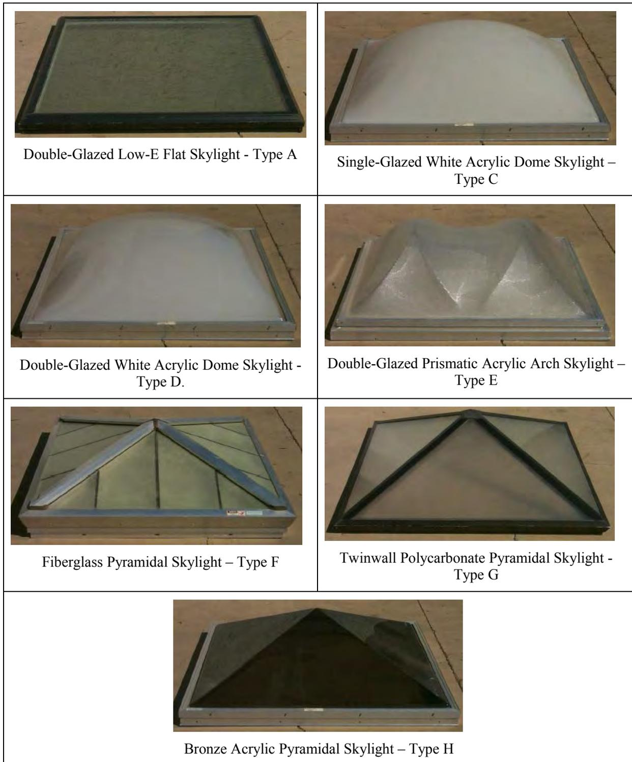
**Figure 15: PIER skylight photometric study test skylight pictures**
