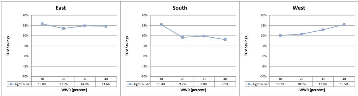
Figure 51: LightLouver TDV energy savings by WWR
