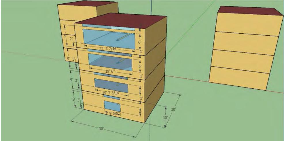
**Figure 2: View window with clerestory prototypes' basic geometry**
