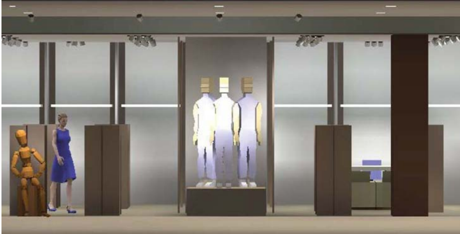
Figure 24: High end retail models A & B. Designer shop 1 80CRI = 2.17W (PASS). Designer shop 2 90CRI = 2.55W (PASS).
