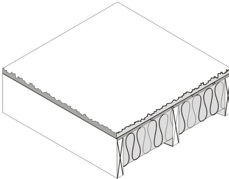
Figure 4.4.1 – Wood Framed Floor with a Crawl Space
