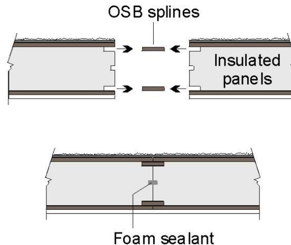
Figure 4.2.4 – SIPS Roof/Ceiling
