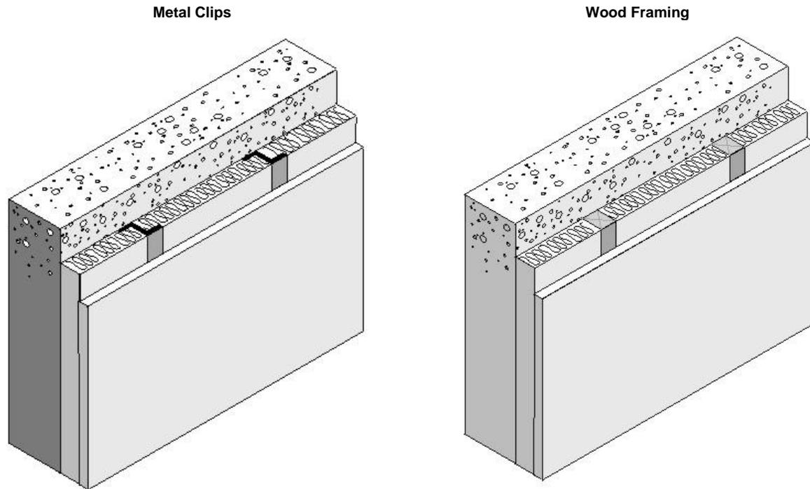
Figure 4.3.14 – Interior or Exterior Insulation Layers
