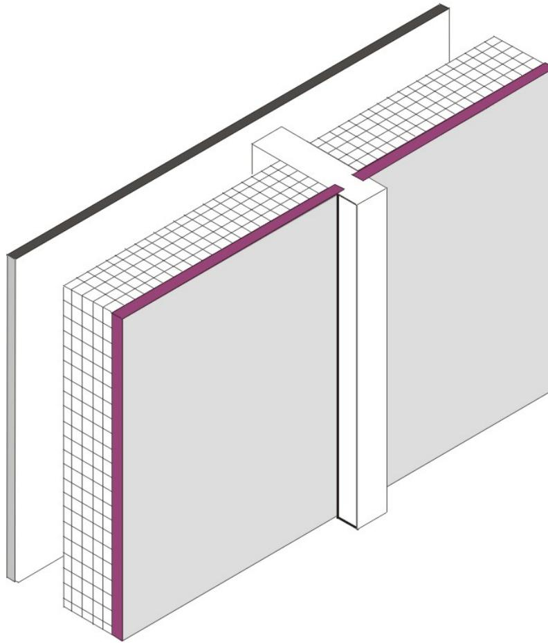
Figure 4.3.8 – Spandrel Panel
