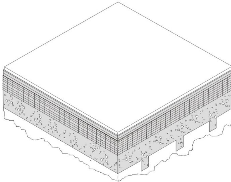
*Figure 4.2.7 – Span Deck and Concrete Roof*
