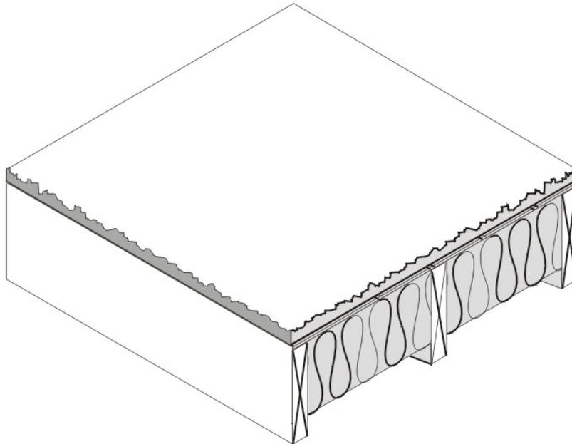
*Figure 4.4.2 – Wood Framed Floor without a Crawl Space*
