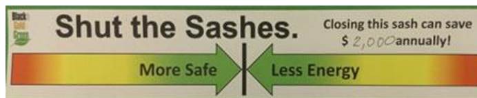
Figure 3. Sash sticker adapted by Purdue University from University of California sticker for horizontally closing sashes, which are not addressed by auto closers.
