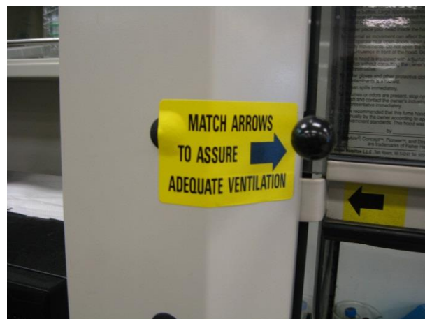
Figures 1a & 1b. Fume hood inspection stickers which may lead to inappropriate operation.
