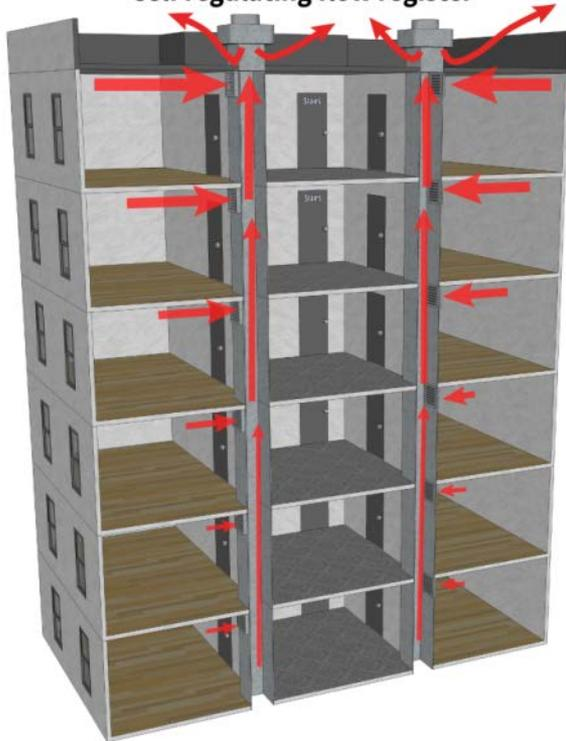
Central exhaust system *with* self regulating flow register
