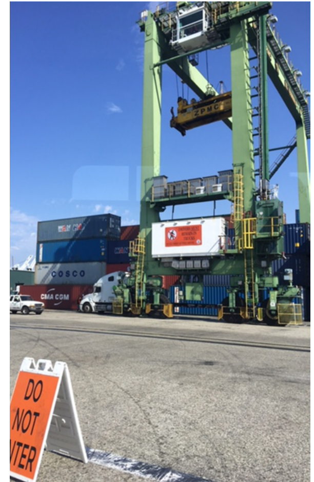
Rubber-Tired Gantry Crane
