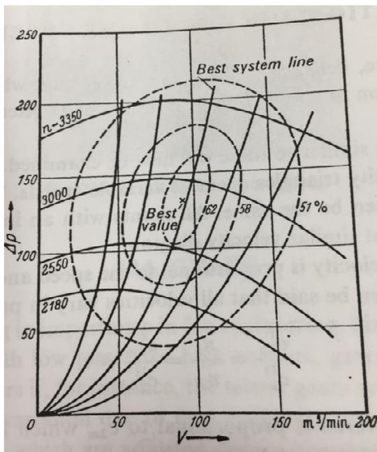
Figure 1 – Fan Curves at Various Speeds Showing Efficiency Change
