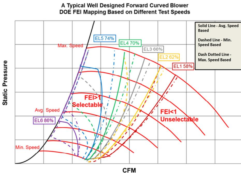
Figure 2 – Fan Map for Various Speeds of Test and Effect on Compliance
