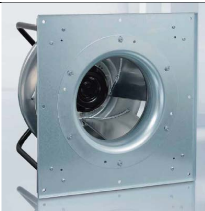
Motorized plenum fan including inlet bell, plate for separation of suction and pressure side, and mounting structure.
