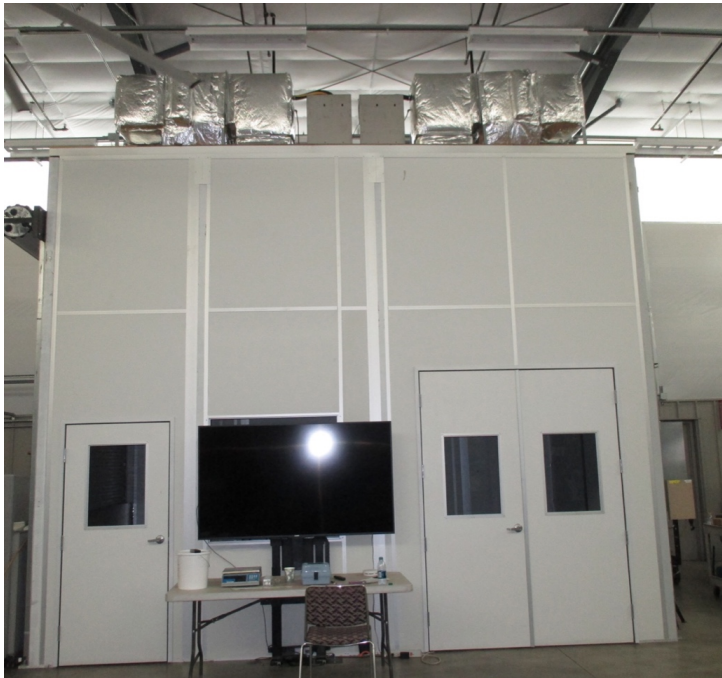
PG&E ATS humidity-controlled and temperature-controlled chamber
