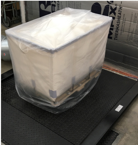
Figure 5.1 Measuring the weight of a laundry cart on a floor scale
