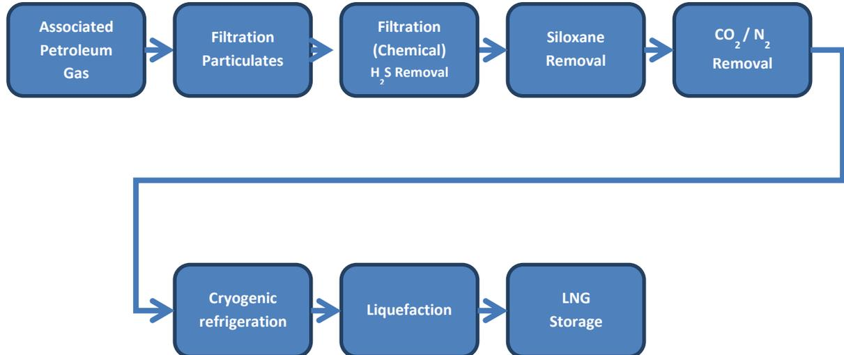
Figure 3: Net Zero LNG™ Process Diagram
