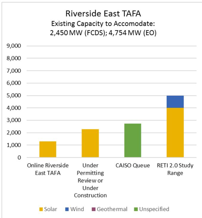
Figure A-8: Riverside East TAFE Existing and Proposed Renewable Energy and Available Transmission Capacity
