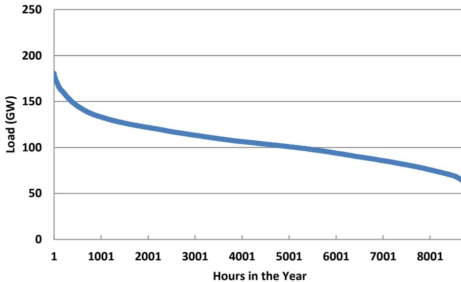
**Figure 7 PJM 2026 Load Duration Curve**
