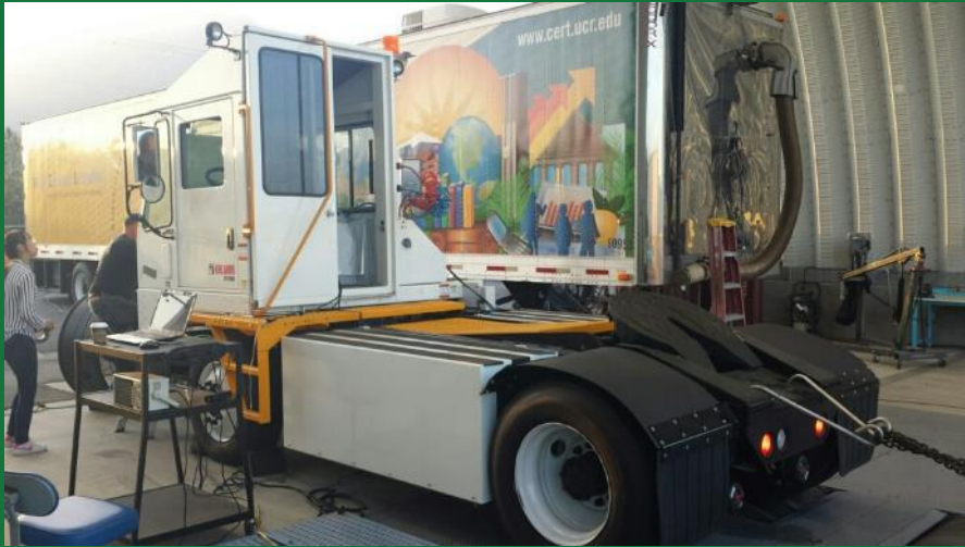
TransPower electric tractor being tested on chassis dynamometer at UC Riverside, 2014
