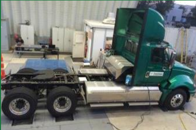
TransPower electric truck being tested on chassis dynamometer at UC Riverside, 2014
