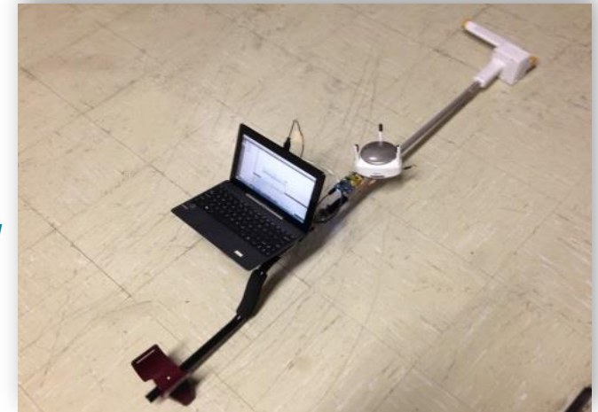
Prototype of handheld methane detector (December 2014)
