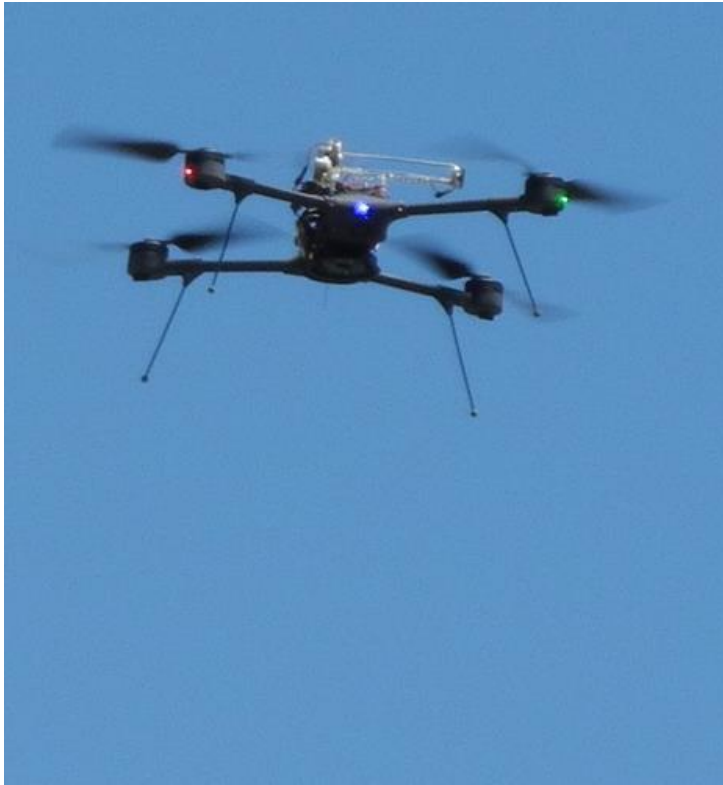
JPL methane detector mounted on a small quadrotor
