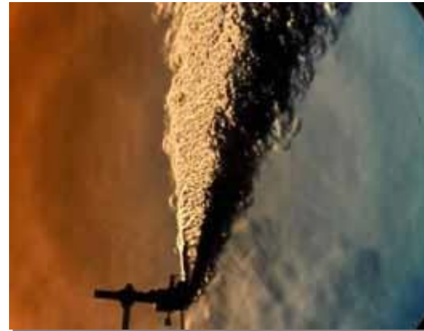
Lab Schlieren image of helium flow
