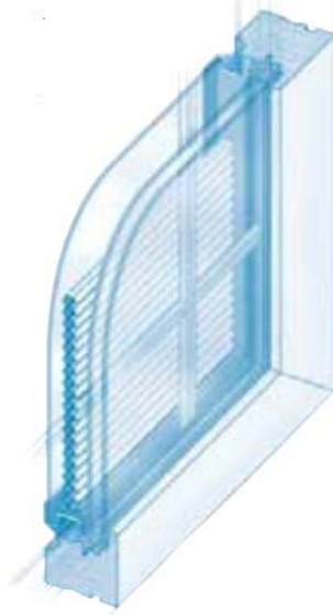
Figure 3-6-5— Example of Dynamic Glazing Type - Integrated Shading System Source: NFRC Dynamic Glazing Products Fact Sheet
