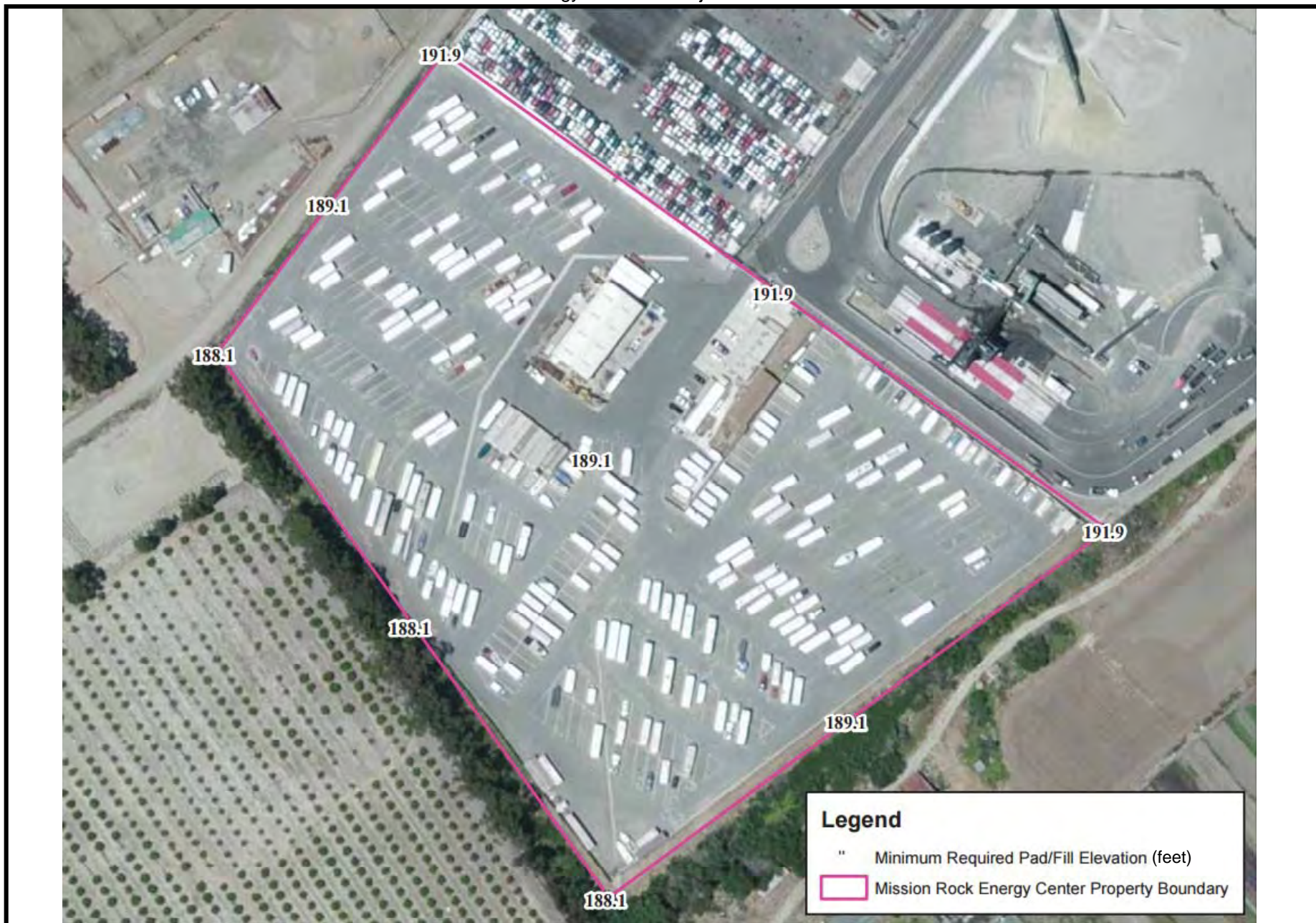
SOIL & WATER RESOURCES - FIGURE 5 Mission Rock Energy Center – Project Site Final Elevations
