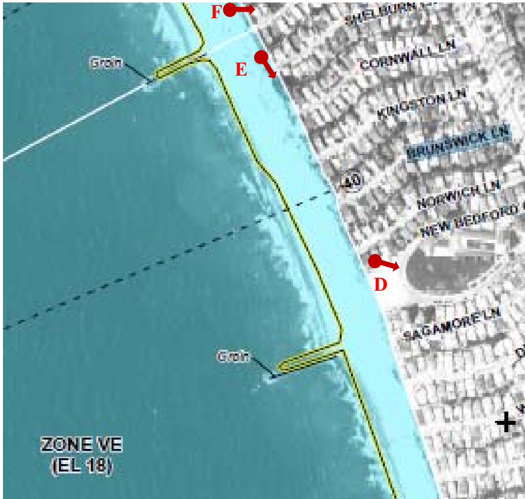
Figure 3B. FEMA Preliminary FIRM map at Pierpont 100 year event, No sea level rise. Flooded area shown in lighter blue. Red arrows indicate approximate location (dot) and orientation of photo. Letters correspond to the ground photo figures for the site.
