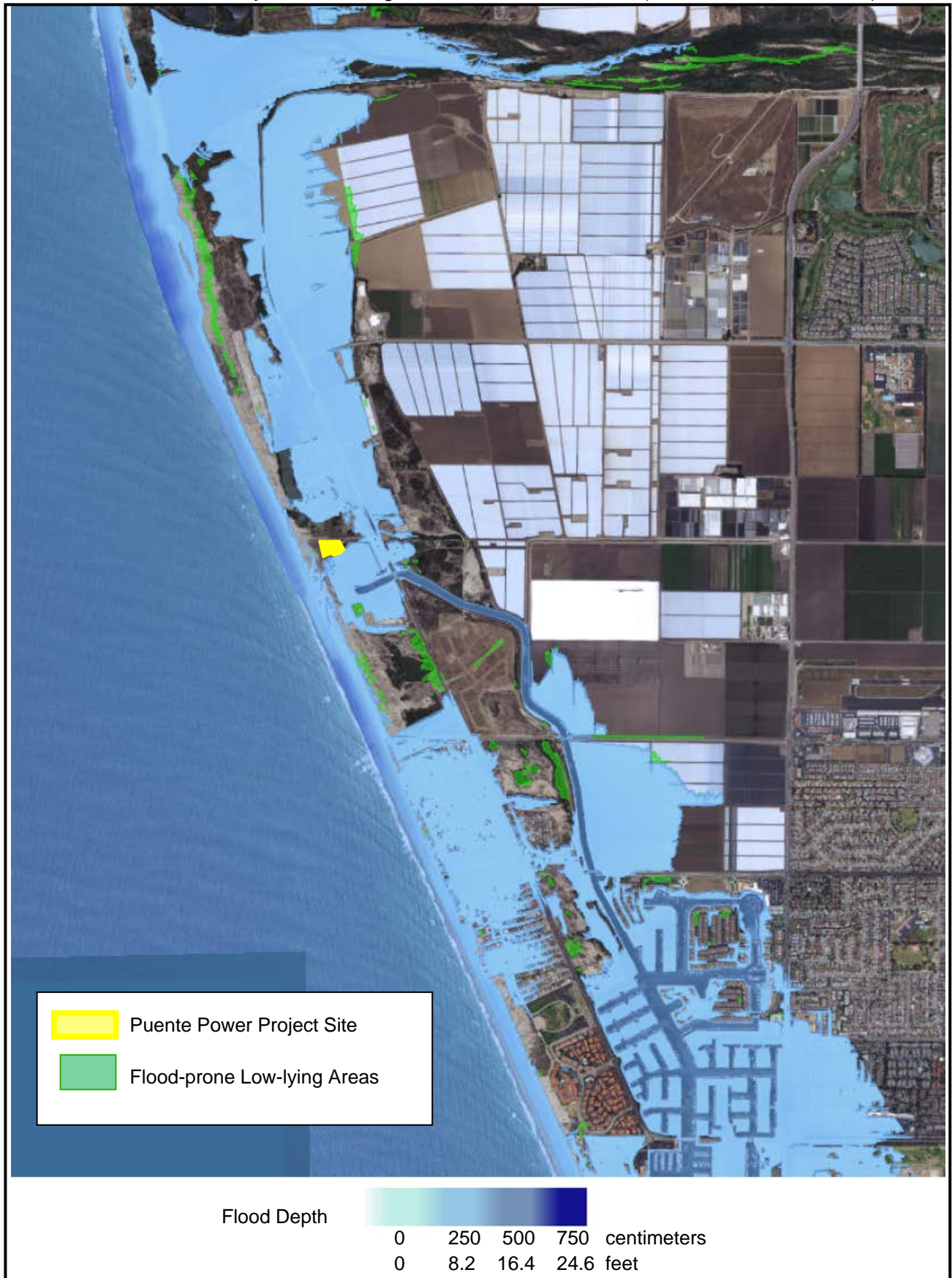
SOIL & WATER RESOURCES SUPPLEMENTAL TESTIMONY - FIGURE 9 Puente Power Project – Flooding Extent of 100-Year Event (Sea Level Rise 6.6 feet)
