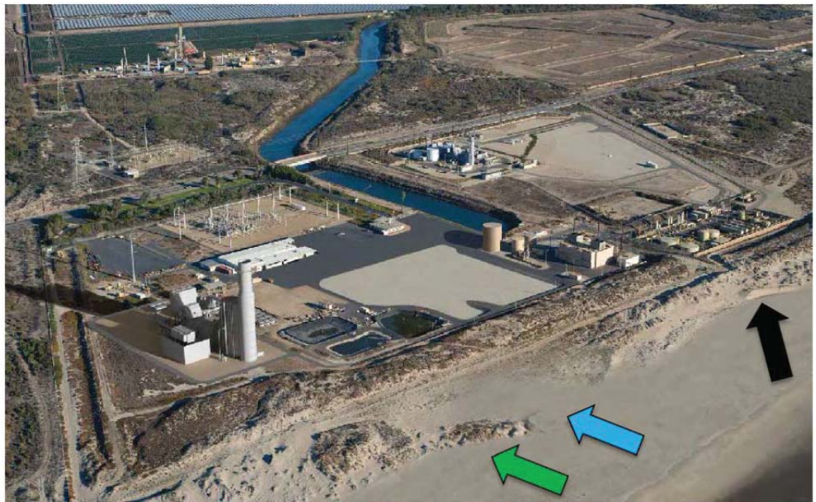
20 Figure 2. Photo from FSA showing view of Puente site with an artistic rendering to show a potential 21 post-construction removal of the existing outfall structure. The black arrow indicates recent dune 22 erosion and the blue arrow shows area of recent wave overtopping to the access road. The green arrow 23 shows part of the area of substantial dune erosion depicted in Figure 3.
