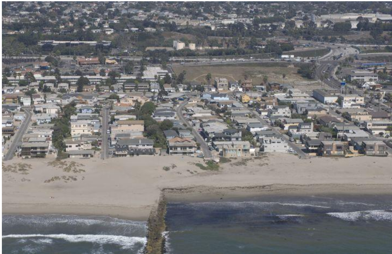
Figure 1. Groin at Pierpont Beach trapping sand to the north (left side of picture), note offset in wet dry line on either side of the groin. Photo courtesy California Coastal Records Project
