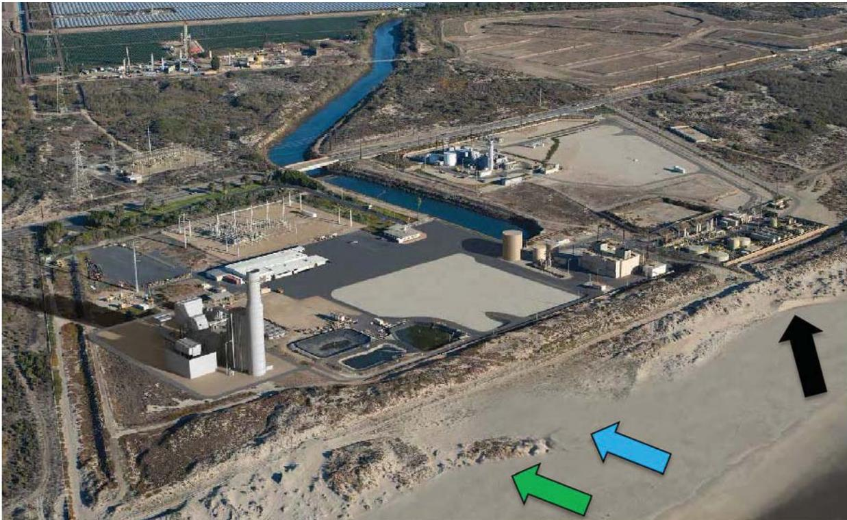
Figure 2. Photo from FSA showing view of Puente site with an artistic rendering to show a potential post-construction removal of the existing outfall structure. The black arrow indicates recent dune erosion and the blue arrow shows area of recent wave overtopping to the access road. The green arrow shows part of the area of substantial dune erosion depicted in Figure 3.
