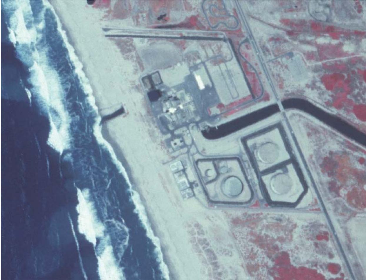
Figure 7. 1984 Color infrared air photo. The photo shows dune erosion fronting the entire site associated with the largest historical storm event, erosion appears most severe in the northern portion of the site.
