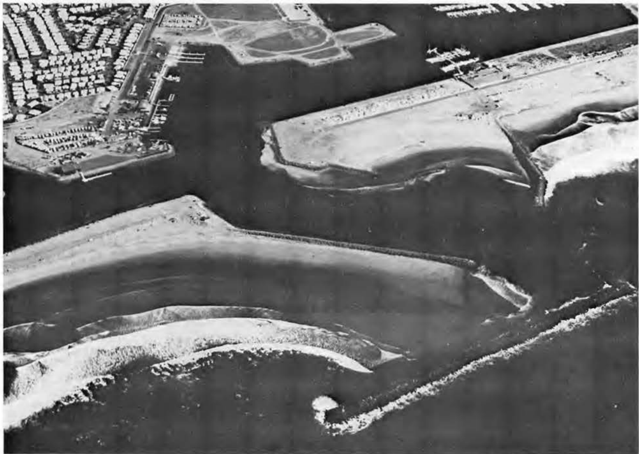
Fig. 3. Aerial photograph of Ventura Marina as of January 1976. Note that the upcoast sand trap in the lee of the detached breakwater is almost completely filled. (Photo by courtesy of the Ventura Port District).
