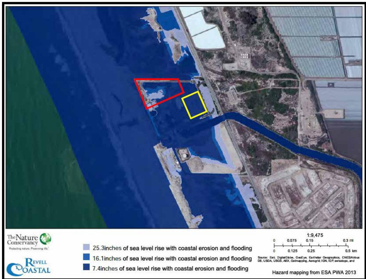
Figure 11. Combined coastal hazards by 2060 for all sea level rise scenarios
