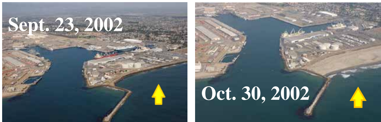
Figure 6. Beach width pre (A: September 23, 2002 ) and post dredging (B: October 30, 2002) downcoast of Port Hueneme (photos courtesy of California Coastal Records Project)
