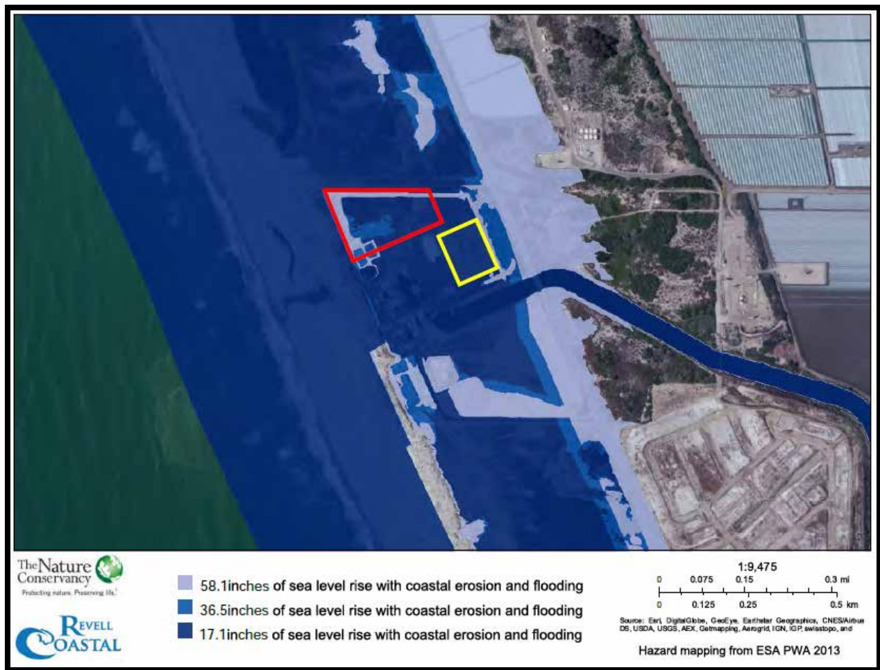
Figure 12. Combined coastal hazards by 2100 for all sea level rise scenarios
