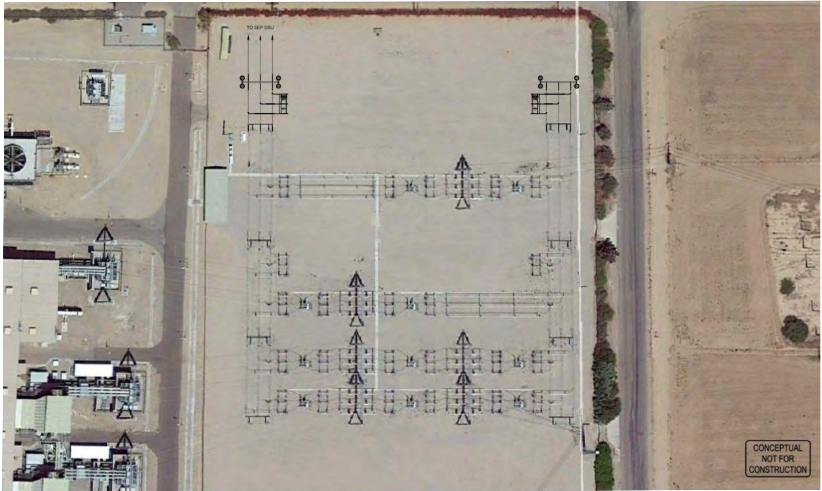
FIGURE 2-5 Electrical 161-kV General Arrangement Buck Termination Diagram Sonoran Energy Project Riverside County, California
