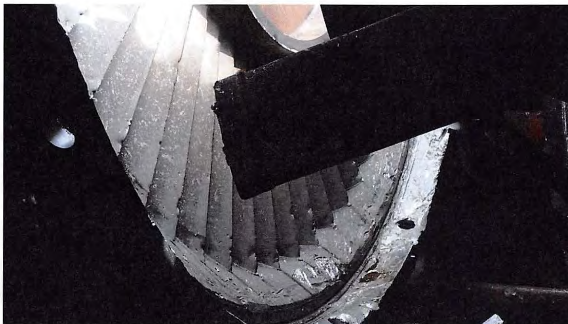
Figure 5. Another view of the damaged turbine blades
