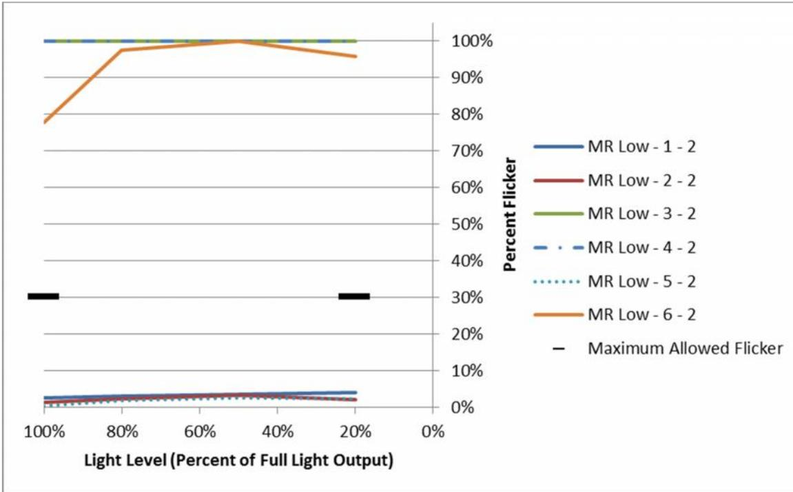
Figure 6 shows that low voltage MR lamps can vary widely in their Percent Flicker levels. These results were confirmed in round-robin testing. Two out of the five lamps had extremely low flicker (less than 5 Percent Flicker). This shows that it is possible to achieve low flicker with a small bulb size, though some lamps exhibit significant flicker.
