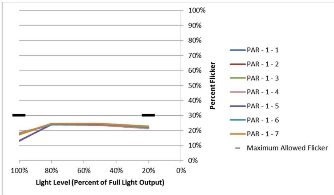
**Figure 2: Percent Flicker (Filtered <200 Hz) vs. dimming level for MR Line 2, all 7 configurations**
