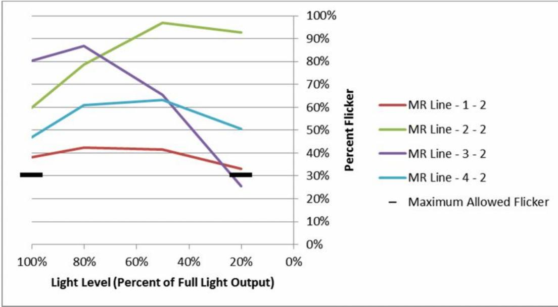
Figure 5 shows that none of the four line voltage MR lamps passed the reduced flicker operation requirements in configuration 2. In fact, none of the line voltage MR lamps meet the California flicker requirement in any of the seven configurations tested.
