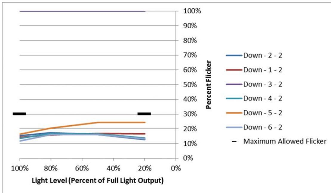
Figure 8 indicates that five out of six of the LED downlights pass the flicker test easily and the one source that fails the test fails poorly with 100 percent flicker. This suggests that even without a flicker test method or standard, much of the downlight market can easily meet the flicker standard, though there are still sources sold with very high flicker levels.
