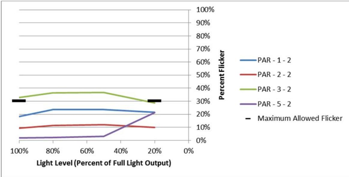
Similarly, Figures 4 through 9 show the results for the other lamp types. As mentioned above, because each of the seven dimmer/number of lamp configurations produced similar results, one configuration (configuration 2) was chosen to demonstrate the results for each lamp.
