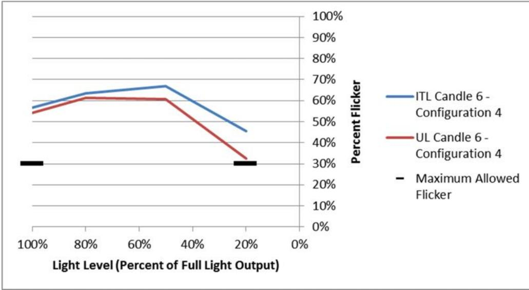
**Figure 17: Round robin test results by lab (filtered <200 Hz) for MR Line 2, configuration 4**
