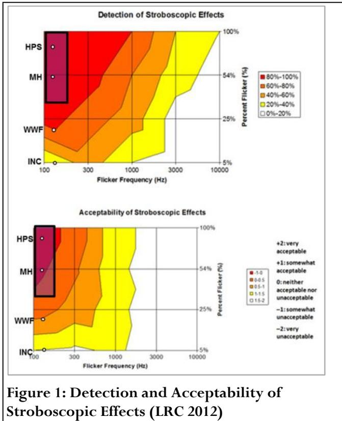
**Figure 1: Detection and Acceptability of Stroboscopic Effects (LRC 2012)**
