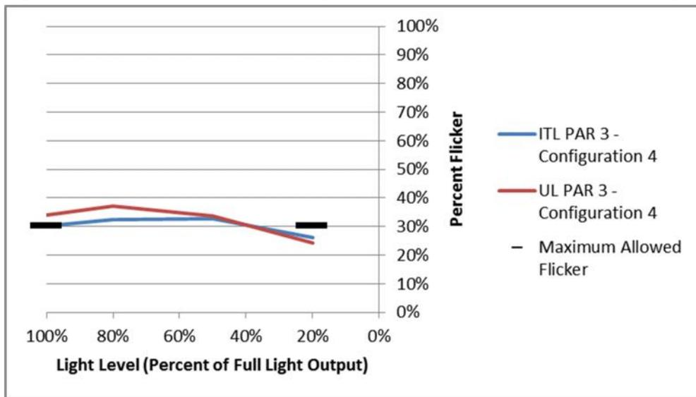
Figure 15 illustrates the problematic situation of where testing with one lab would find that the product fails the test method and another lab would find that it passes. For this particular lamp at full output the UL results measured 34.1 percent flicker and the ITL results were 30.2. Actually both fail but the ITL results are very close to passing.
