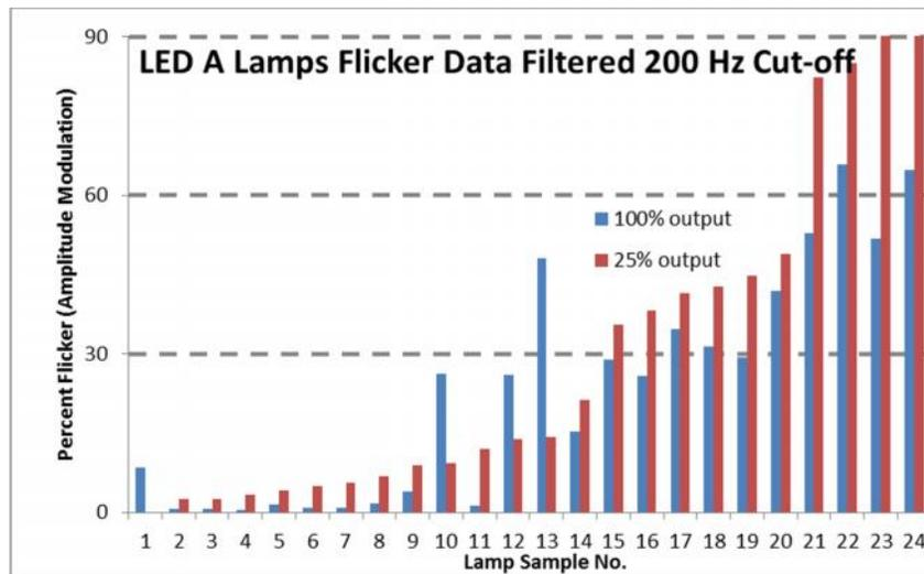
**Figure 3: Filtered Flicker Test Data for 25 LED A-lamps (filtered flicker proposed for CA standards)**
