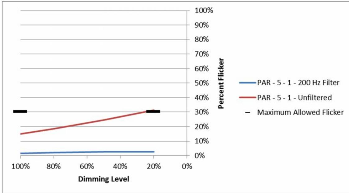
**Table 5: Overall average Percent Flicker for filtered and unfiltered data at 100% and 20% light output**
