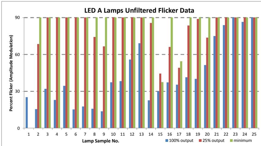
**Figure 4: Unfiltered Flicker Test Data for 25 LED A-Lamps (unfiltered flicker not proposed for CA standards)**
