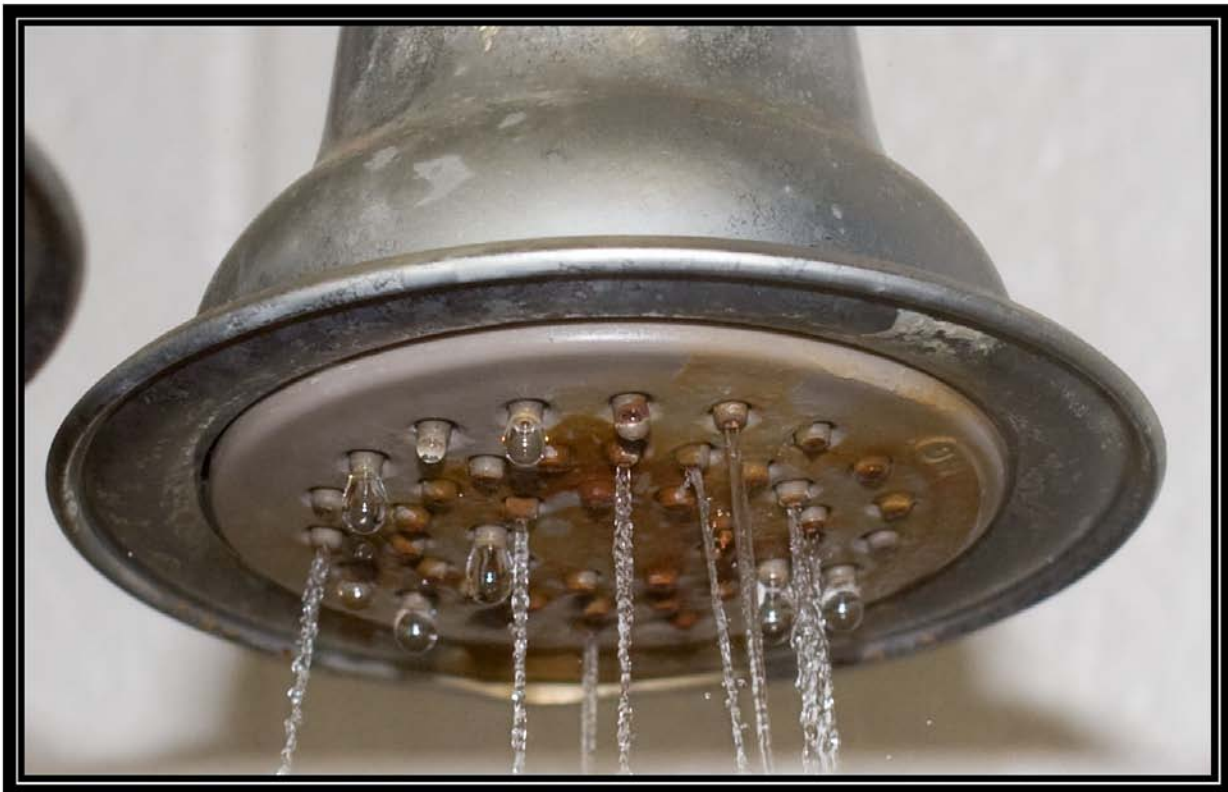
Figure 6-10D. Showerhead 10 on seventh day of testing with hard well water (28 grains per gallon) showing spray pattern. Battelle testing for Water Quality Association. May 1, 2009
