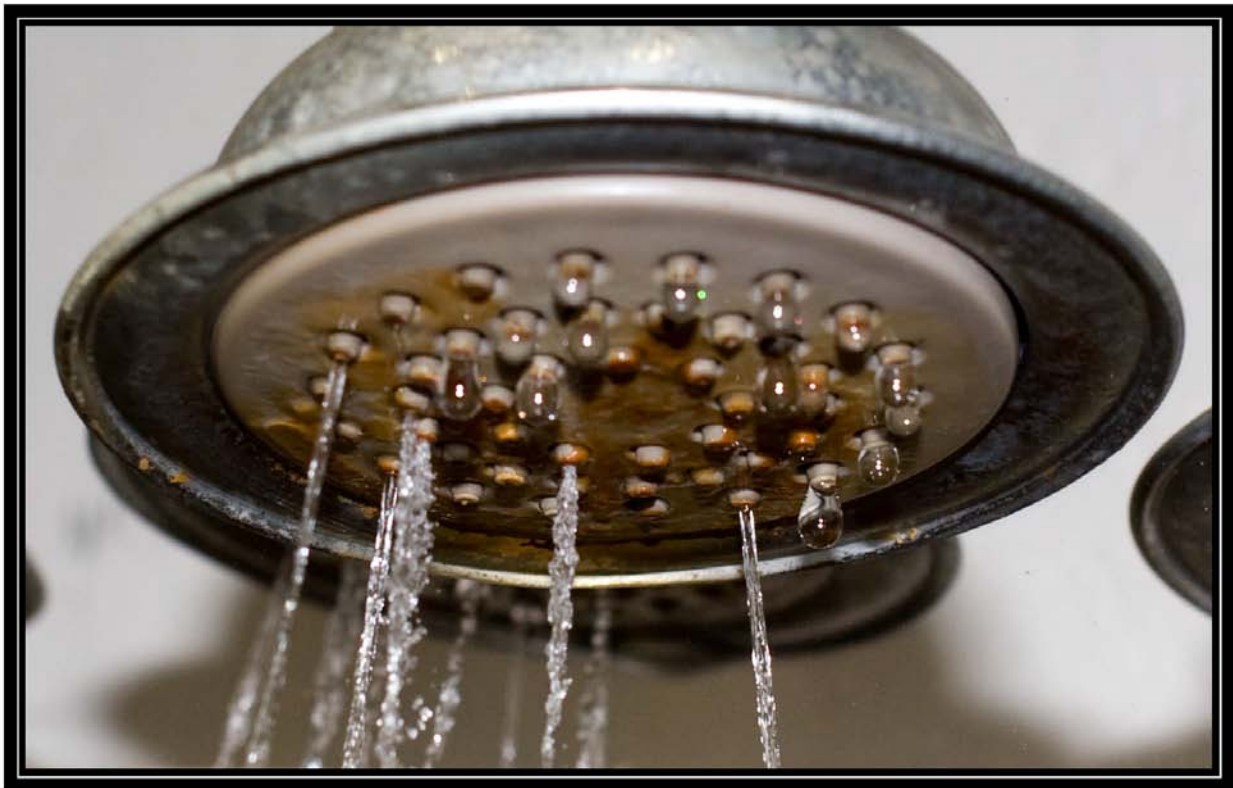
Figure 6-7D. Showerhead 7 on seventh day of testing with soft well water (28 grains per gallon) showing spray pattern. Battelle testing for Water Quality Association. May 1, 2009
