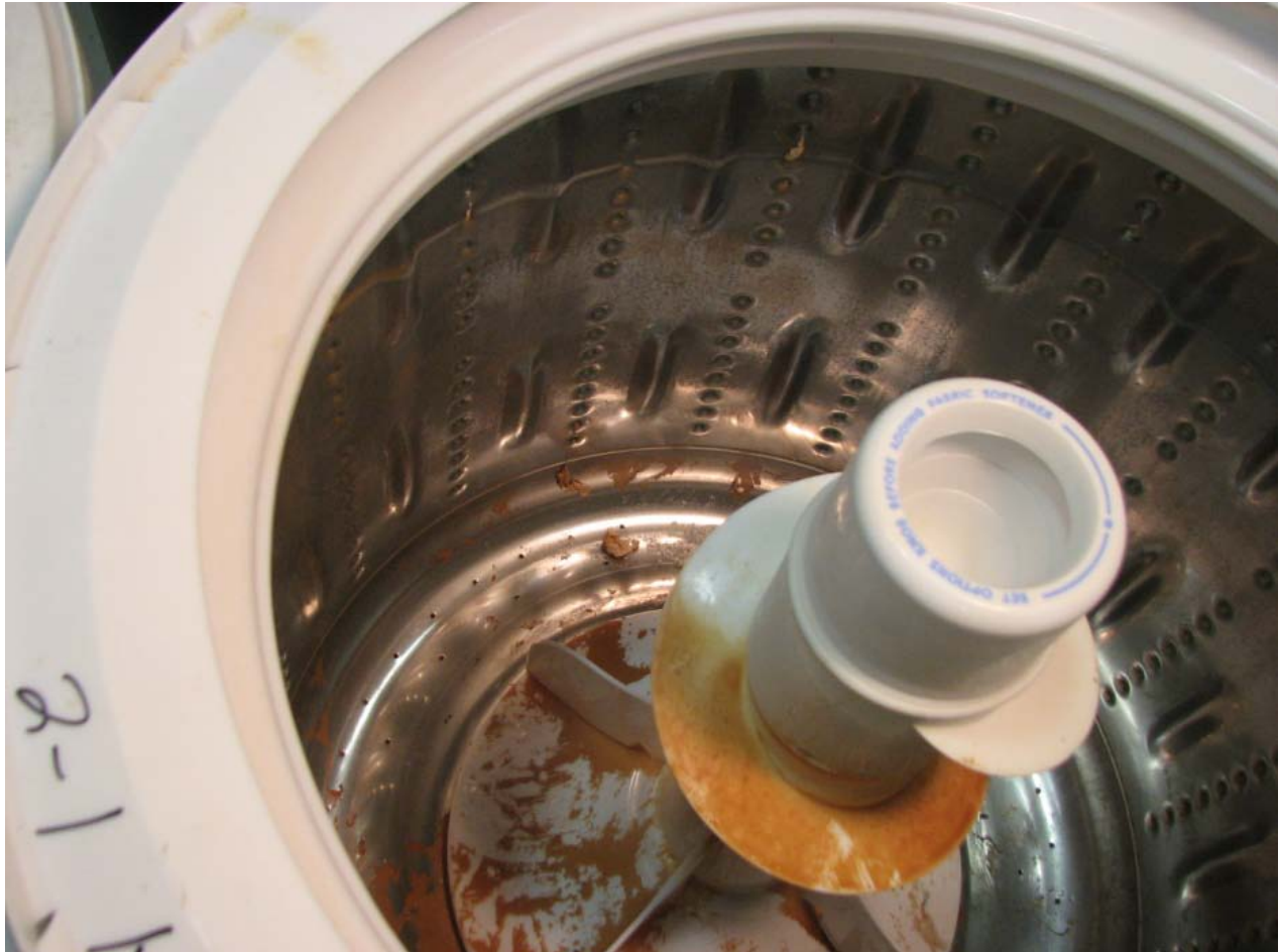
Figure 5-27. Drum of the laundry washer using unsoftened water had significant water scale buildup on all of the interior surfaces.
