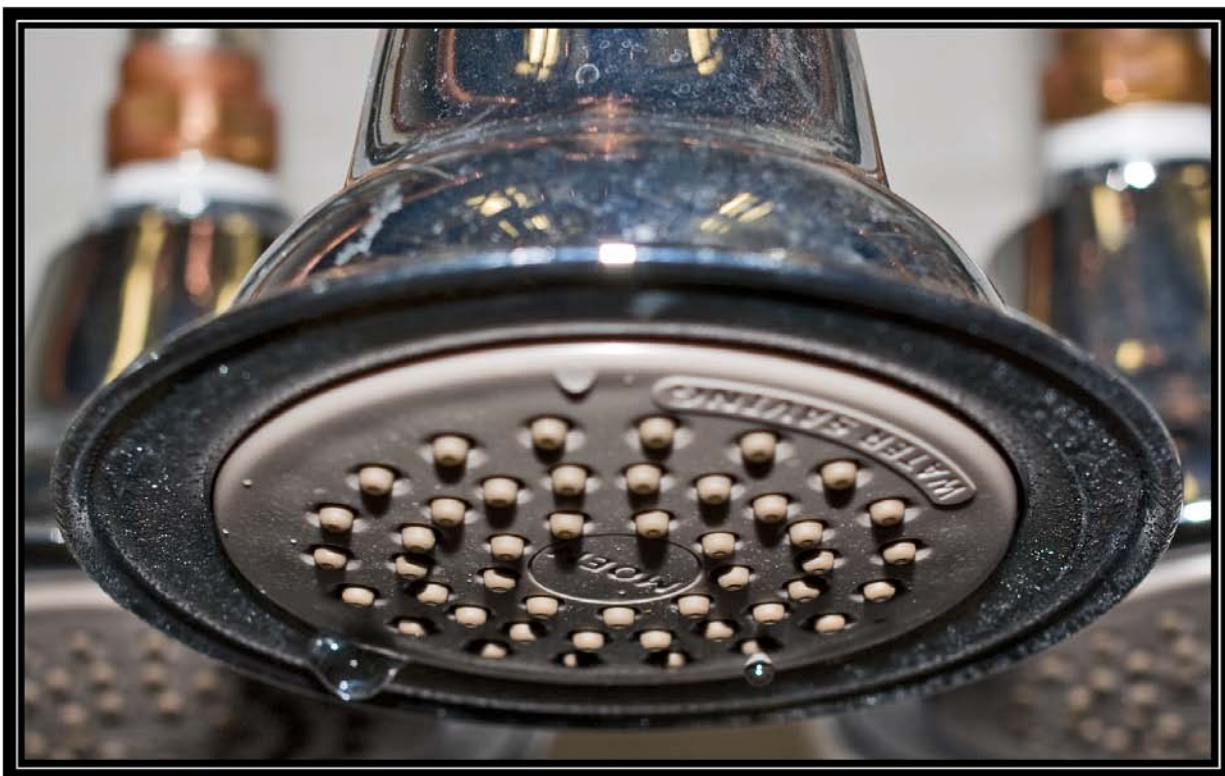
Figure 6-1A. Showerhead 1 on fourth day of testing with softened well water (<1 grains per gallon) showing condition of nozzles. Battelle testing for Water Quality Association. April 28, 2009
