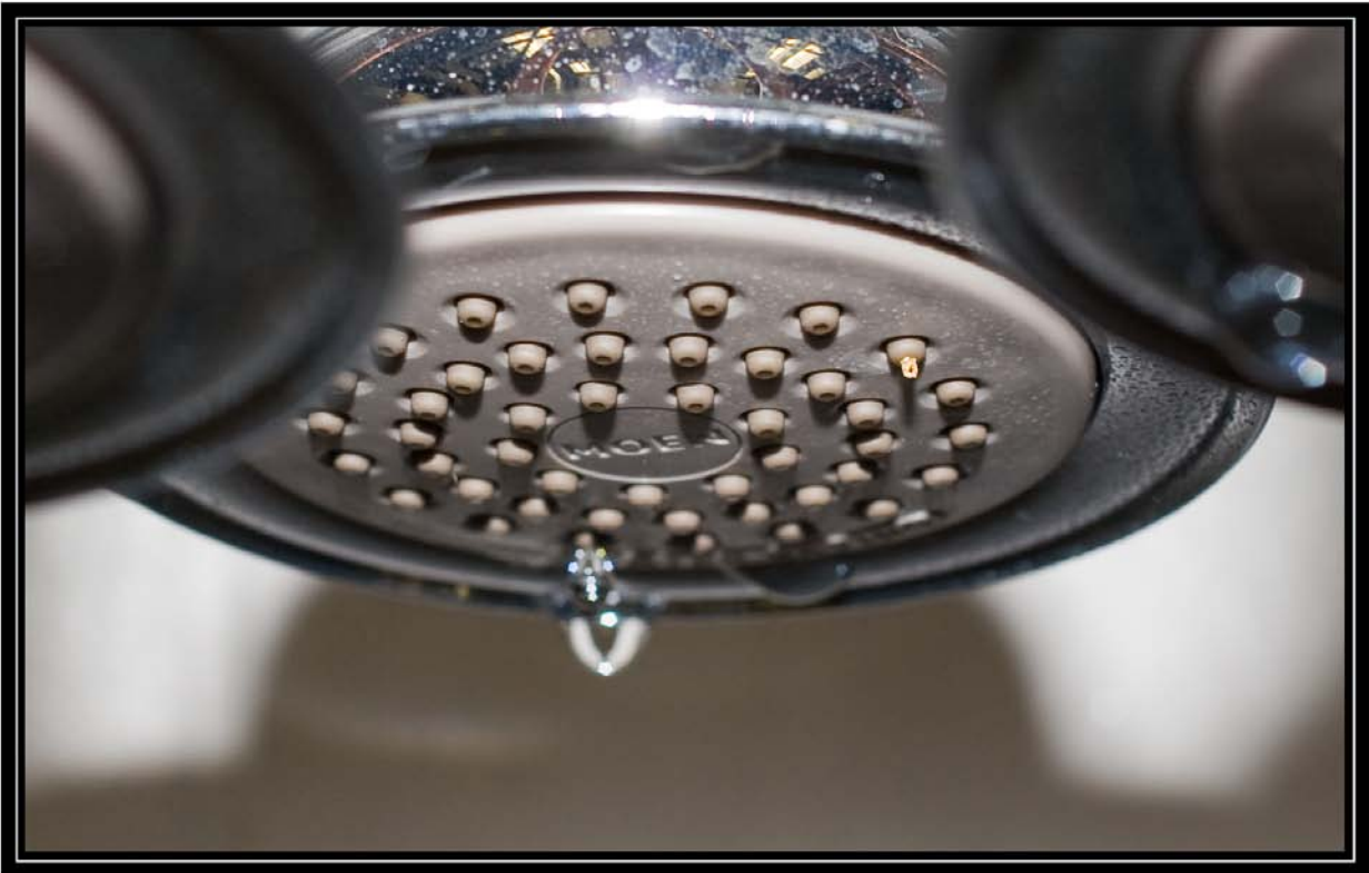
Figure 6-4A. Showerhead 4 on fourth day of testing with softened well water (<1 grains per gallon) showing condition of nozzles. Battelle testing for Water Quality Association. April 28, 2009
