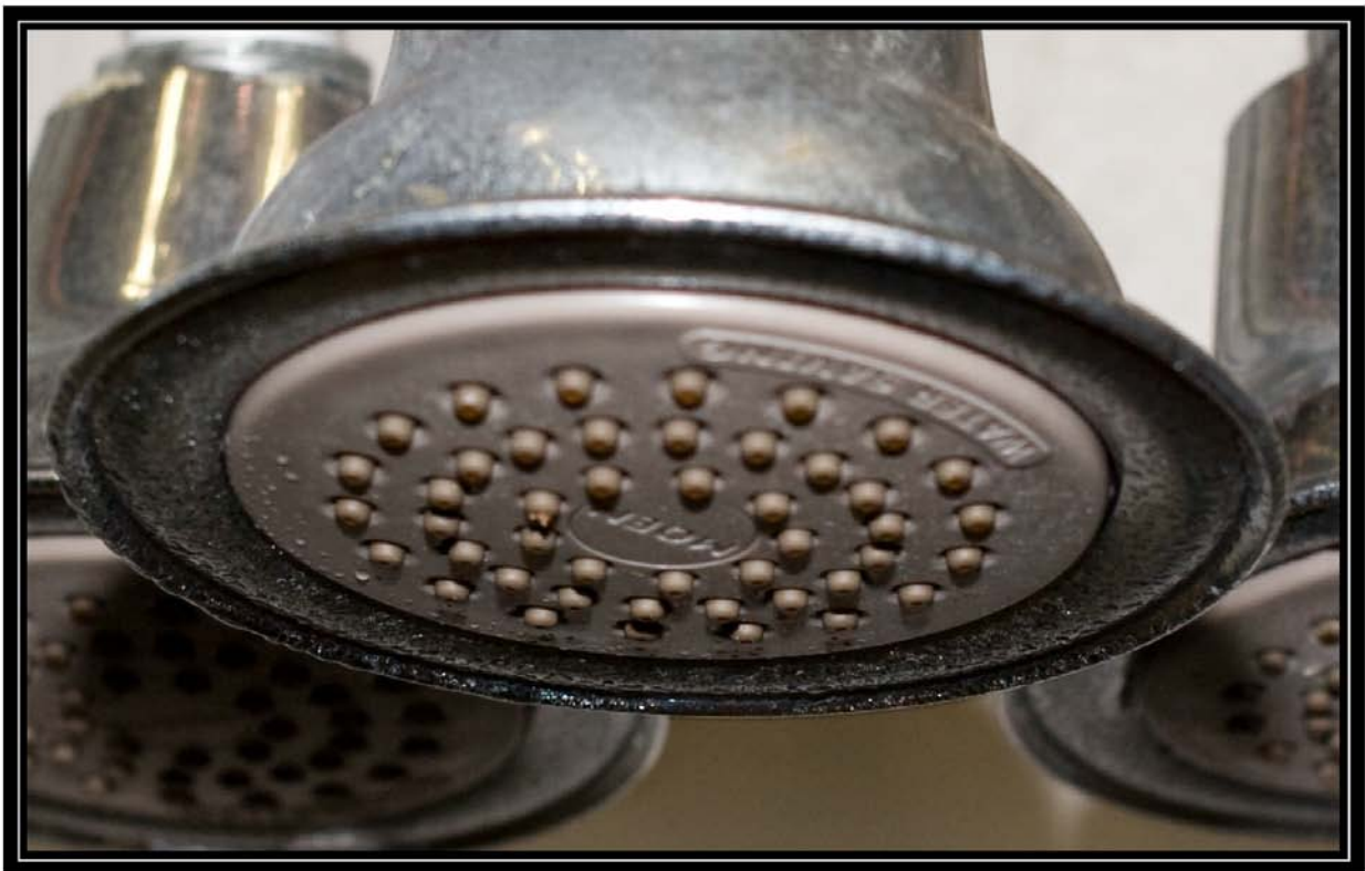
Figure 6-2C. Showerhead 2 on seventh day of testing with soft well water (<1 grain per gallon) showing condition of nozzles. Battelle testing for Water Quality Association. May 1, 2009
