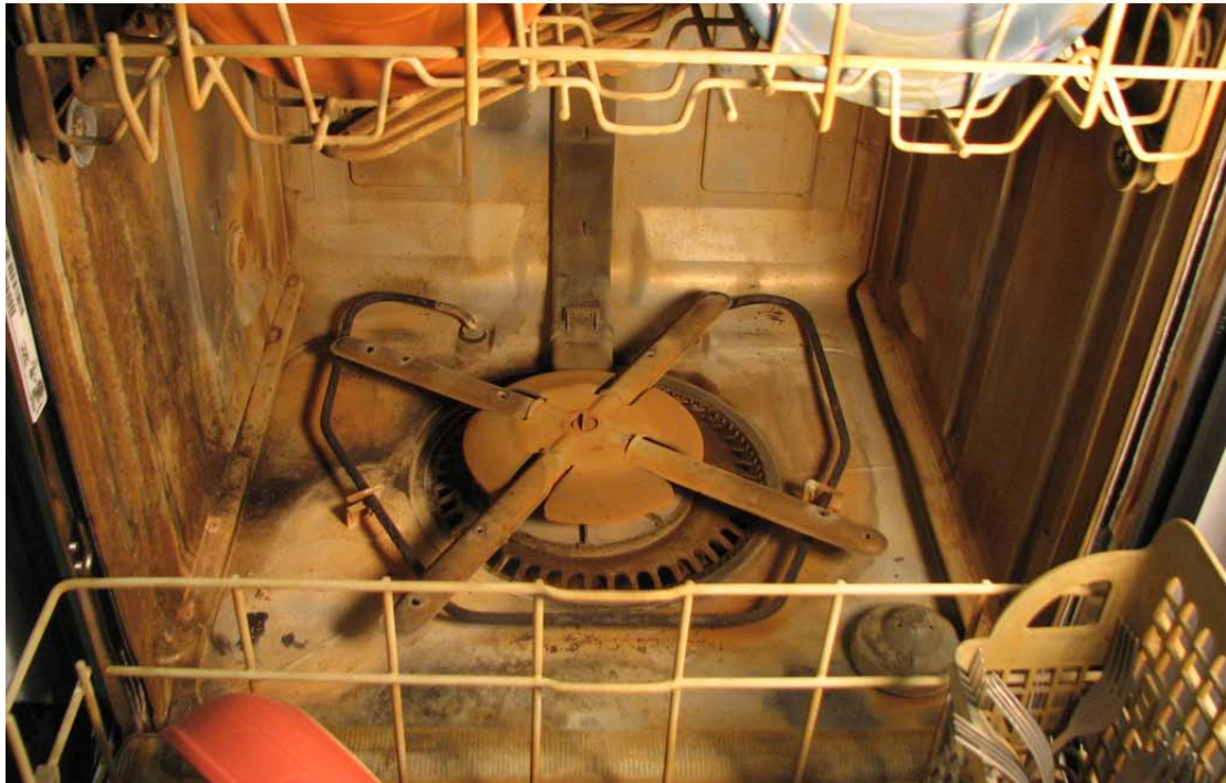
Figure 5-25. Photos showing condition of dishwasher at the end of 30 days using unsoftened water.
