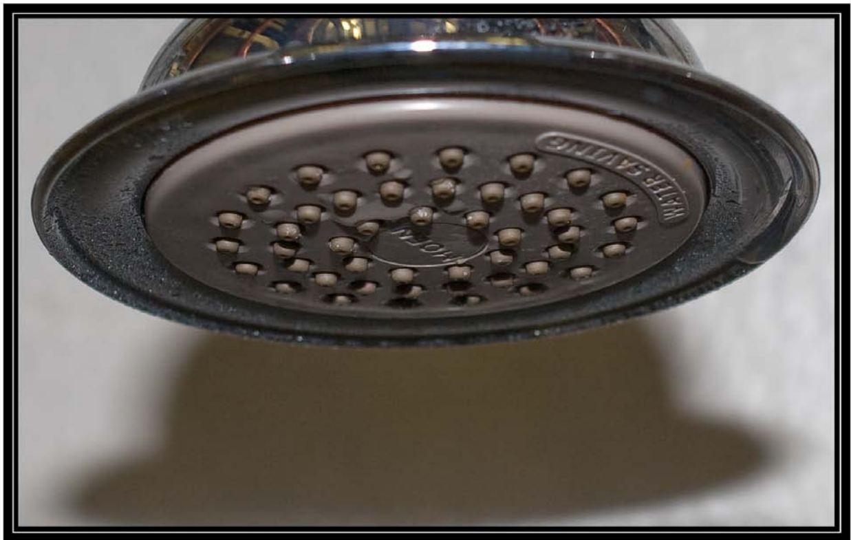
Figure 6-5A. Showerhead 5 on fourth day of testing with softened well water (<1 grains per gallon) showing condition of nozzles. Battelle testing for Water Quality Association. April 28, 2009
