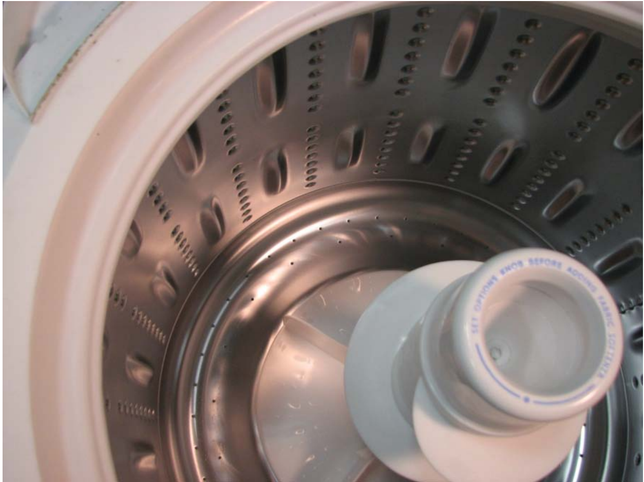
Figure 5-26. Drum of the laundry washer using softened water was almost completely free from water scale buildup.
