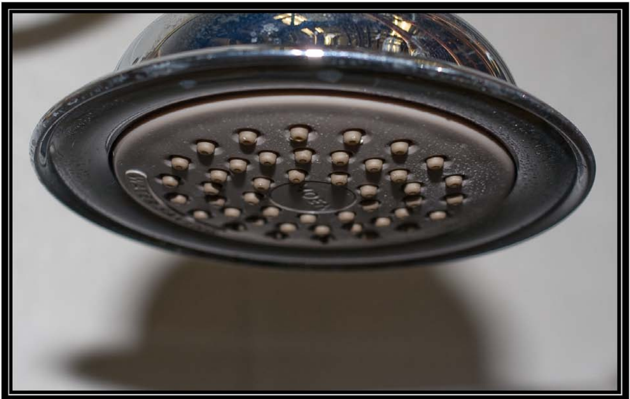
Figure 6-3A. Showerhead 3 on fourth day of testing with softened well water (<1 grains per gallon) showing condition of nozzles. Battelle testing for Water Quality Association. April 28, 2009
