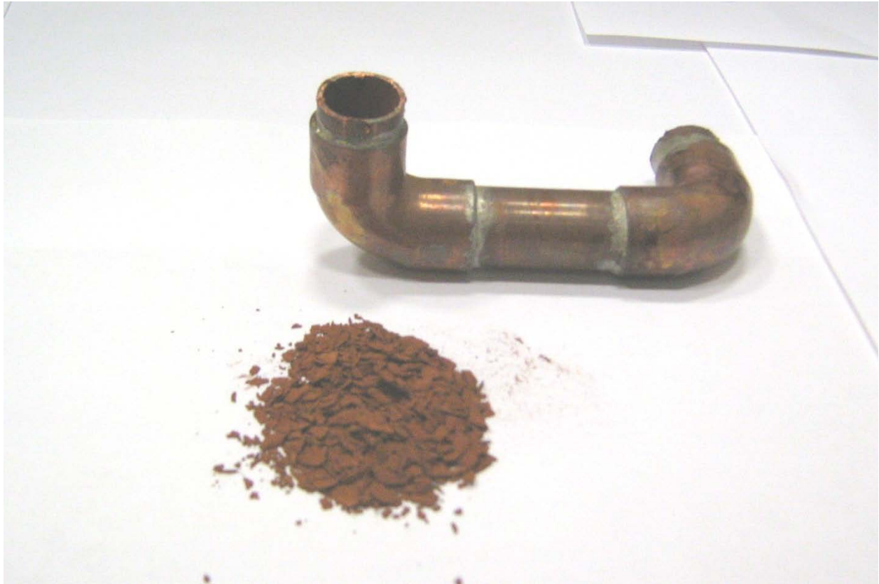
Figure 5-4. Loose scale inside the elbow from the instantaneous water heater on unsoftened water.
