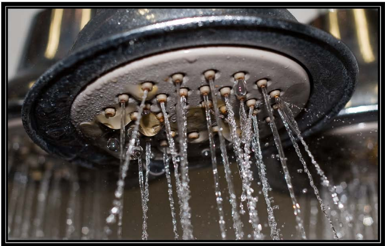
Figure 6-7B. Showerhead 7 on fourth day of testing with hard well water (25 grains per gallon) showing spray pattern. Battelle testing for Water Quality Association. April 28, 2009
