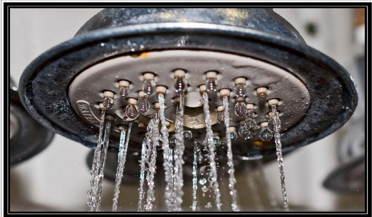
Figure 5-18. Typical spray pattern from one of the showerheads using unsoftened water at the end of the test.
