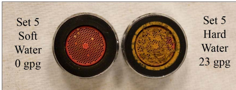
Figure 5-23. Photo showing the Set 5 faucet strainers at the end of the test.
