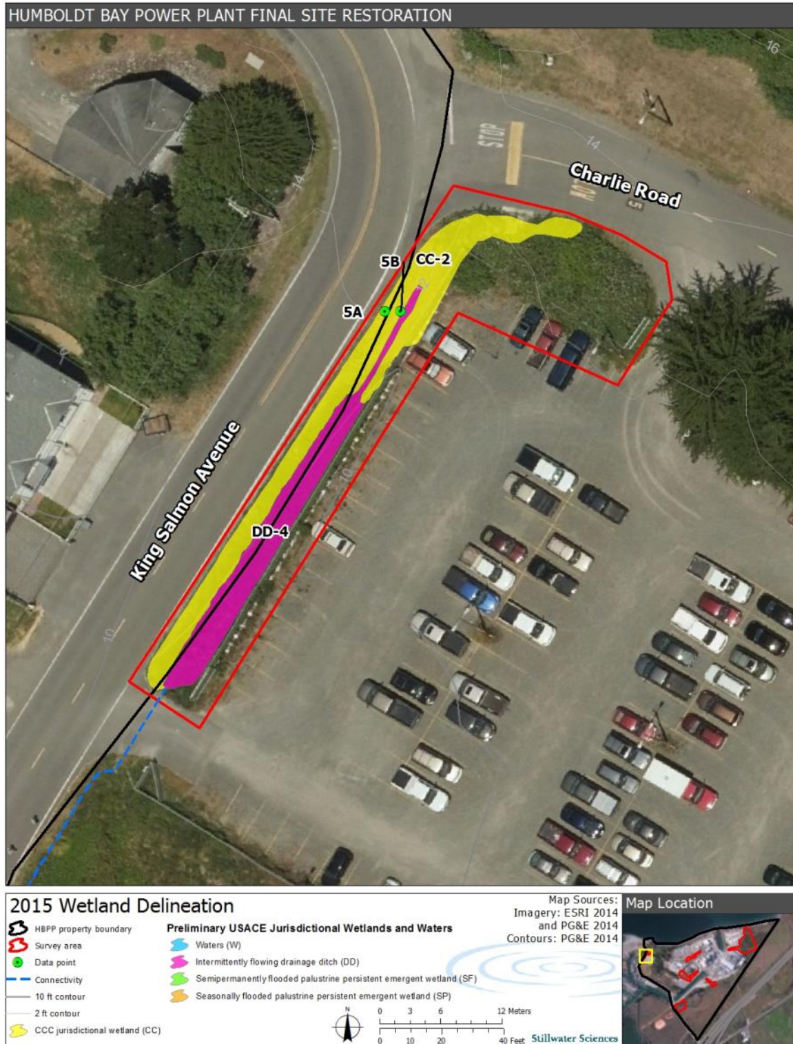
Figure 10. Preliminary waters of the U.S. identified in the Charlie Road Parking survey area.
