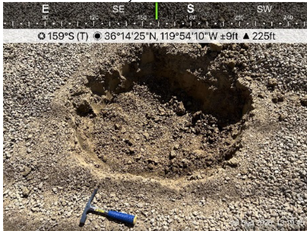
After manually digging was completed. The second hole looked like this as well. Estwing for scale. Brown clay and gravel is present.
