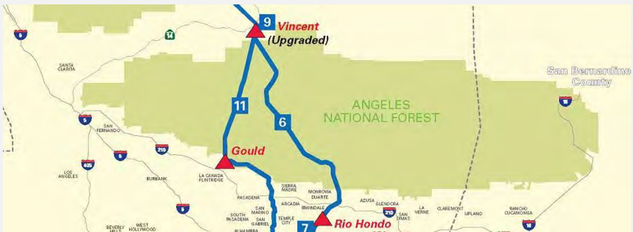
Exhibit 5. SCE map showing the upgraded/replaced transmission line sections completed as part of the Tehachapi Renewable Transmission Project. These upgrades follow the alignment of P19186876 (11 in map).
